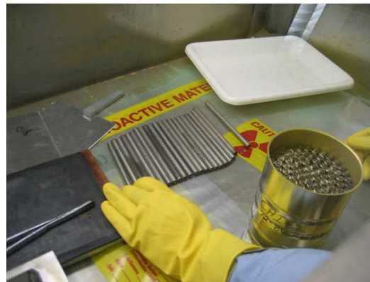
Fig. 5-7. MOX fuel pins of well-known composition were packaged into two cans in known quantities.
