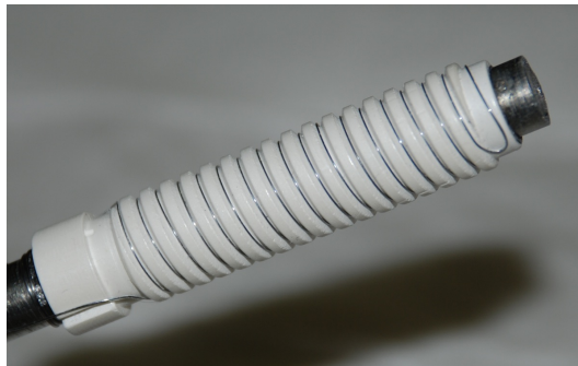
Figure 3.3: Updated heater on the second \text{LaB}_6 cathode.
