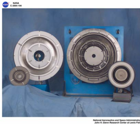
Figure 2.7: Hall-effect thrusters developed by NASA ranging from 3 kW to 50 kW nominal power. Photo courtesy of NASA.
