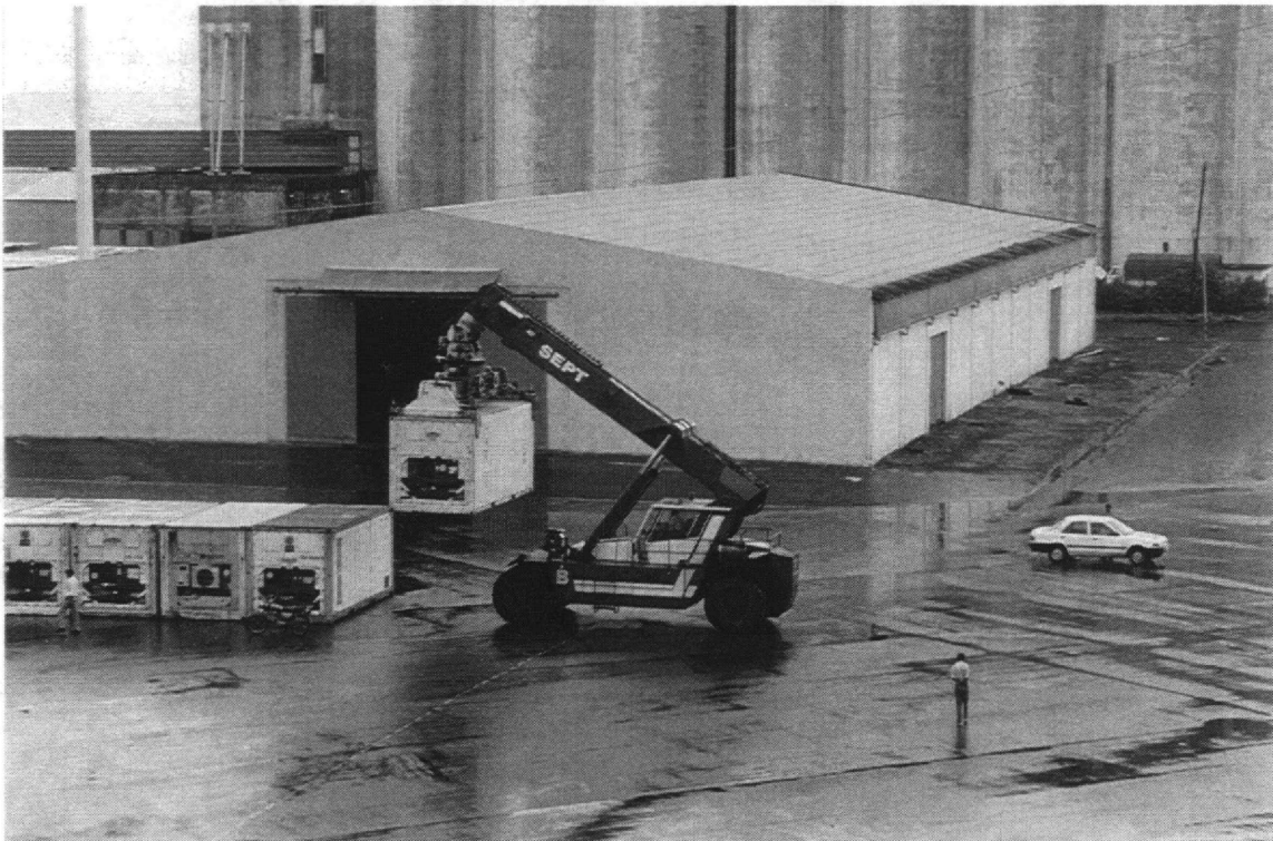
One of three PPM super-stackers places a container. Grain silos are behind.
