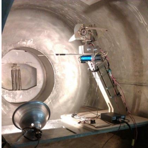
Figure 2.4 Flapping wing test stand in vacuum chamber
