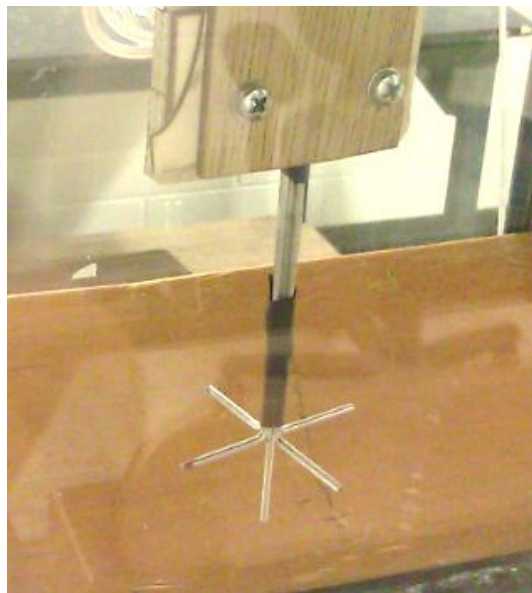
Figure D.4 First gen prop-wash probe geometry
