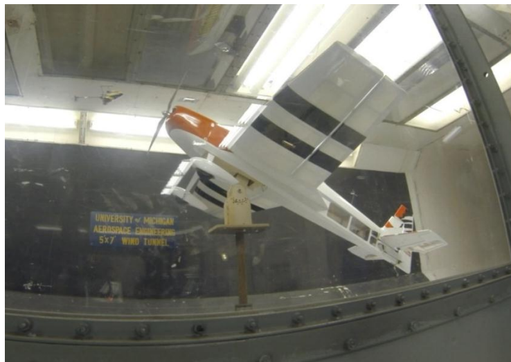
Figure 2.5 Fixed wing test platform with internal force-torque transducer
