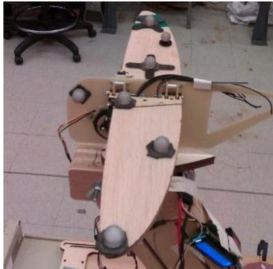
Figure 3.5 Large VICON targets on rigid balsa wings
