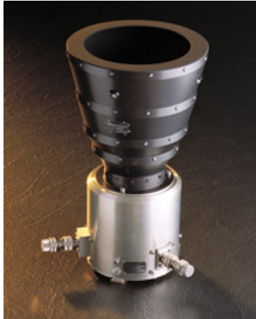
(a) Ball Aerospace CT-633 star tracker, which has a mass of 2.5 kg without the baffle, 13.4 cm diameter, requires 8 W of power, and provides an attitude accuracy of better than 0.01^\circ .
