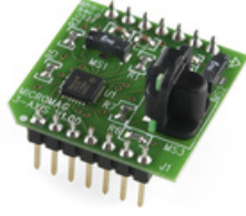
(a) PNI MicroMag3 three-axis magnetometer. The physical dimensions are 2.54 \times 2.54 \times 1.9 \text{ cm}^3 and the sensor requires 1.5 mW.
