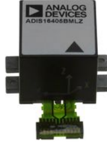
(b) Analog Devices ADIS13405 inertial measurement unit, which includes a three-axis rate gyroscope, three-axis accelerometer, and a three-axis magnetometer. The physical dimensions are 2.3 \times 2.3 \times 2.3 \text{ cm}^3 and the sensor requires 225 mW.
