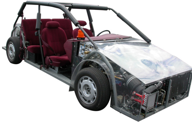
Figure 1.1: Prototype series hydraulic hybrid vehicle developed by the EPA.
