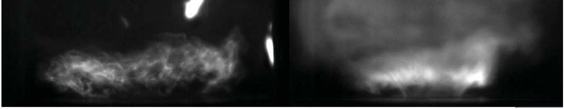
Figure 4.14: Instantaneous flame chemiluminescence images of ethylene ( left ) and 25% H 2 syngas ( right ). Note that there is some flame structure connecting the main portion of the syngas flame brush to the burner. Similar structure is not apparent in the liftoff height for hydrocarbon flames. Air \dot{m} = 282 g/min, \phi = 0.75 .
