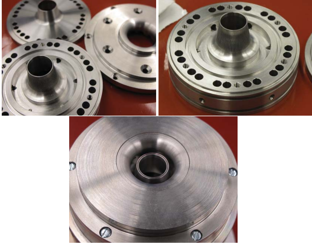
Figure 2.3: Images of the core components of burner and the core assembled.
