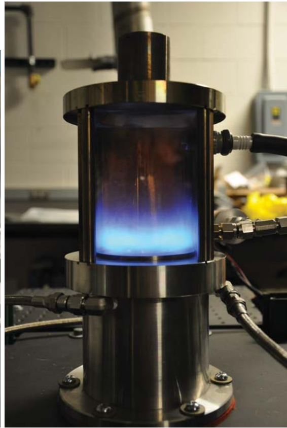
Figure 2.2: Images of the standard GTMC configuration in operation.
