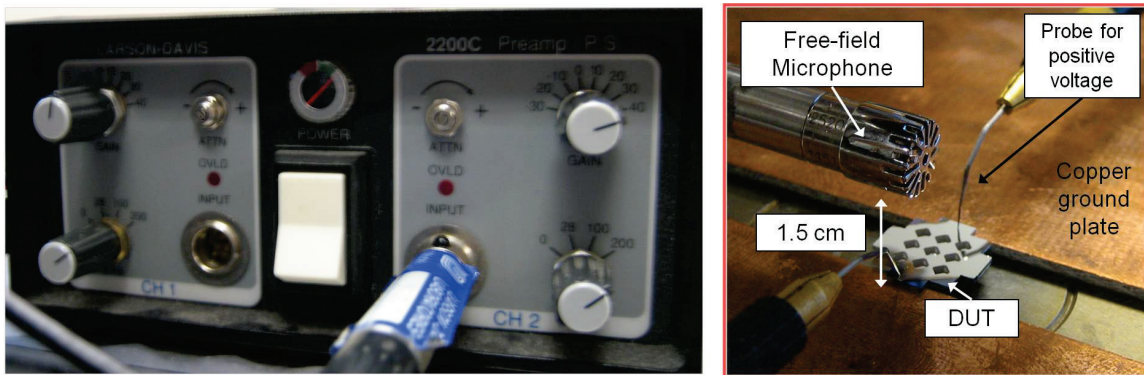
Figure 4-14: (Left) Pre-amplifier for powering the calibrated microphone and (Right) The free-field calibrated microphone placed 1.5 cm away from the DUT.
