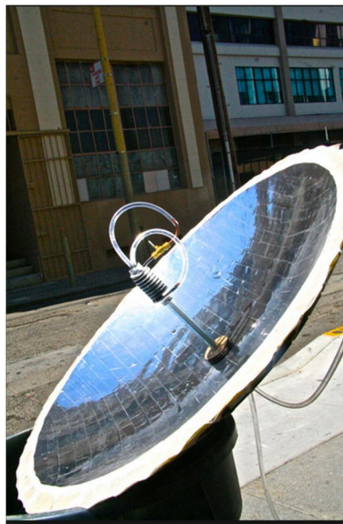
Figure-12: SWH with parabolic dish
