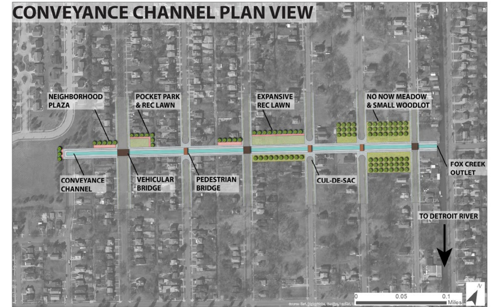
Figure 48: Plan View of Conveyance Channel Replacing the Eastern Portion of Essex Avenue within the Jefferson-Chalmers Neighborhood.
