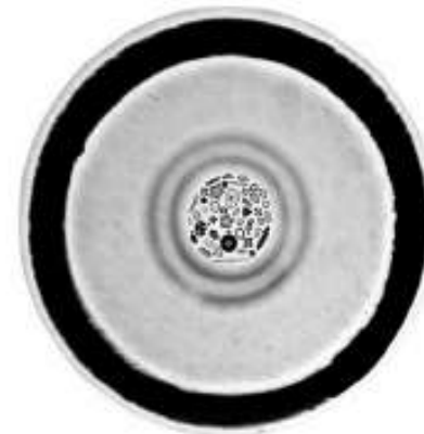
Figure 5. Light-colored guide rings on the rear of the slide and dark India ink ring on the mounting glass to help locate the diatom arrangement. The guide rings are removed when the slide is finished. (Photo copyright retained by author).
