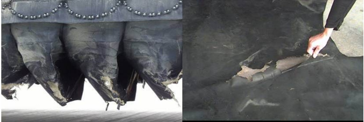
(a) Delamination of first generation LCAC deep-skirt after 100 hours (Lavis, 2009).
