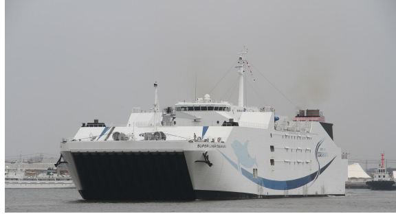
Figure 2.2 Ogasawara Techno-Superliner (TSL), largest surface-effect ship (SES) built to date, 140 m in length.
