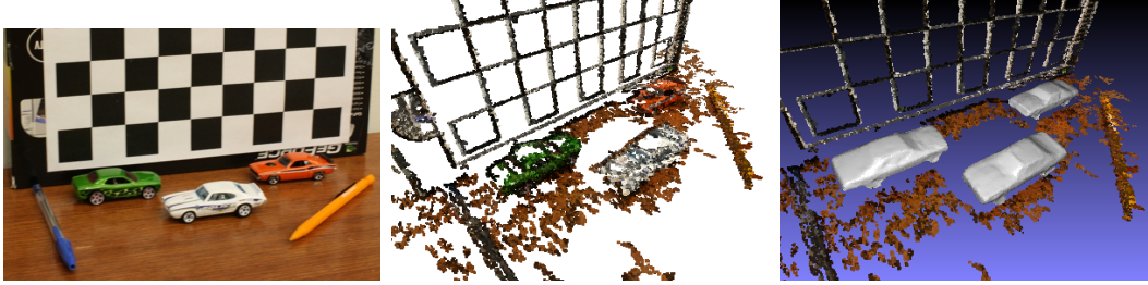
Figure 5.10: Reconstruction of multi-object scenes. (Left) 1 out of 10 input images. (Middle) MVS Furukawa et al. (2010) . (Right) Our reconstruction.
