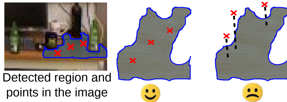
(a) The estimated 3D points (red crosses) should lie on the estimated 3D region (a portion of desk).
