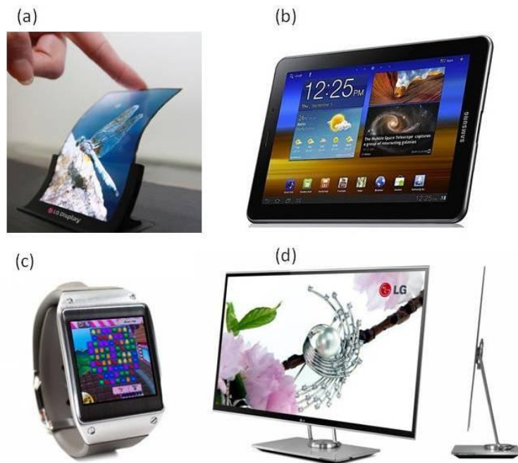
Figure 1.8 (a) A prototype flexible phone from LG, (b) A tablet computer from Samsung, (c) A smart watch from Samsung, (d) A TV from LG. All these electronic devices use OLED displays.
