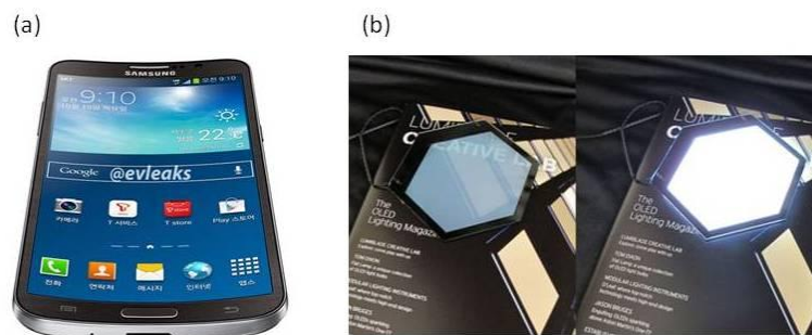
Figure 1.2 (a) Samsung's Galaxy Round smart phone using a curved OLED display (b) A transparent OLED lighting panel manufactured by Phillips
