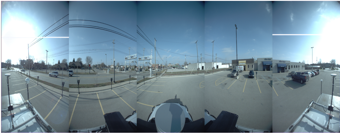
Figure C.5 The distorted images, from the five horizontal sensors of the omnidirectional camera, stacked together.
