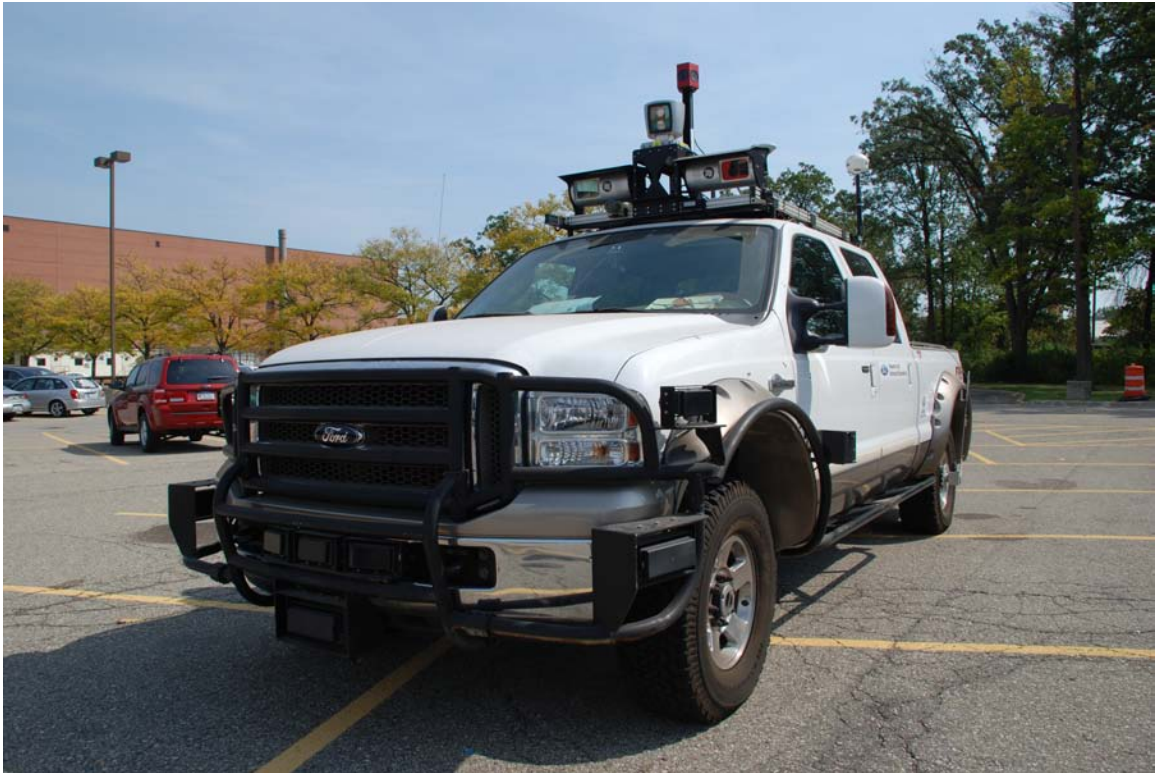
Figure C.1 The Ford F-250 pickup truck with perception and inertial sensors strategically mounted on the vehicle for autonomous navigation research.
