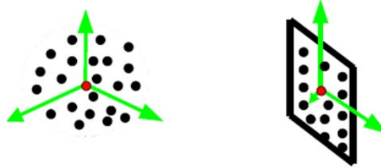
Figure 4.3 Local neighborhood structure of 3D points used in GICP algorithm [146] is captured by the sample covariance matrix. Planar surfaces show two dominant eigen-vectors of the sample covariance matrix (right). Uniformly distributed points show equal eigen-vectors in all three dimensions (left).
