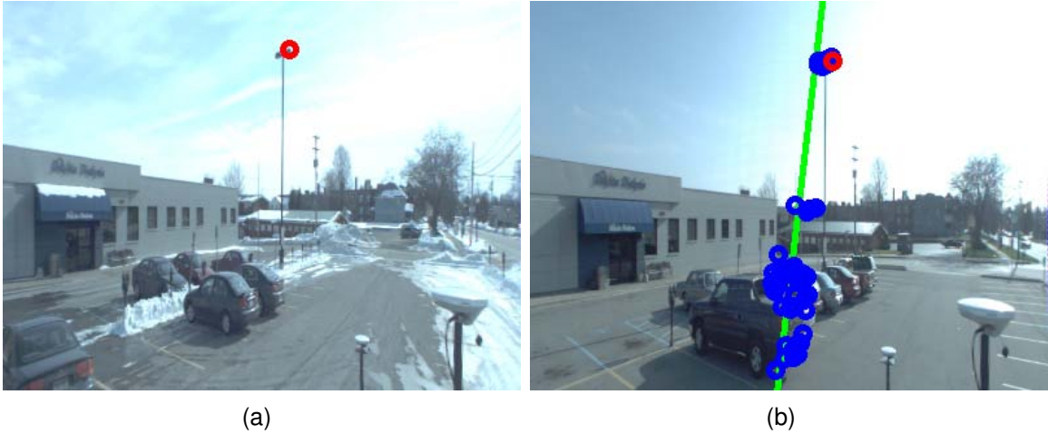
Figure 5.6 The left panel shows a sample codeword (on the lamp-post) extracted from the query image. The right panel shows the epipolar line (green) for the same codeword in the corresponding image from the map. The potential correspondences are marked in blue and the correct correspondence computed based on codeword similarity is marked in red.
