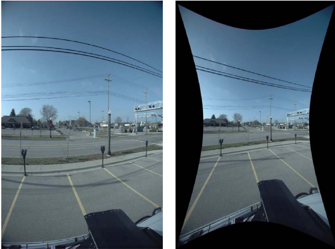
Figure C.6 The left panel shows a spherically distorted image obtained from the Ladybug3 camera. The right panel shows the corresponding undistorted image obtained after applying the transformation provided by the manufacturer.
