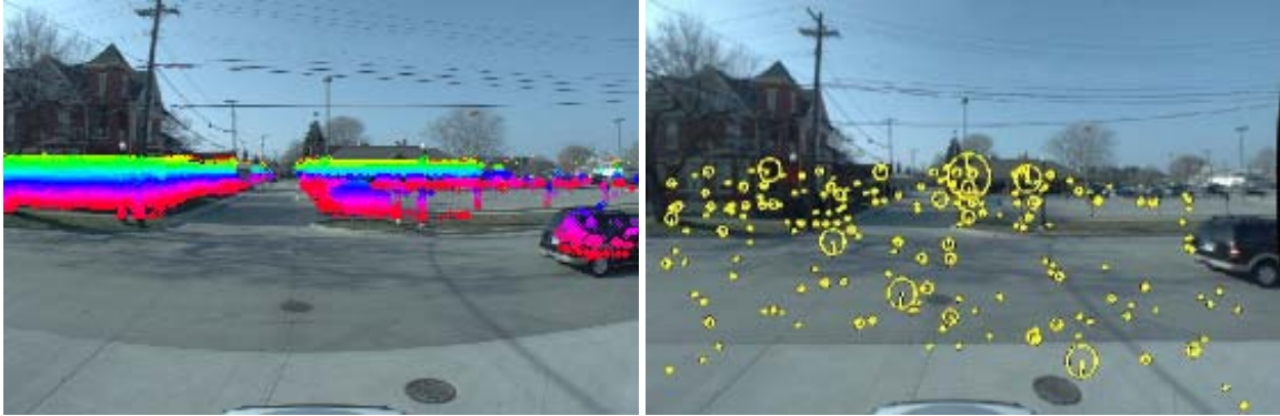
Figure 4.4 The co-registered camera and lidar data is shown below. The left panel shows the 3D points projected on the image plane, only points above the ground plane are shown here. The right panel shows SIFT features corresponding to the 3D points projected on the image plane. The points high up (e.g., on the facades of building) generally do not have a corresponding 3D point because of limited vertical field of view (FOV) of the laser scanner.
