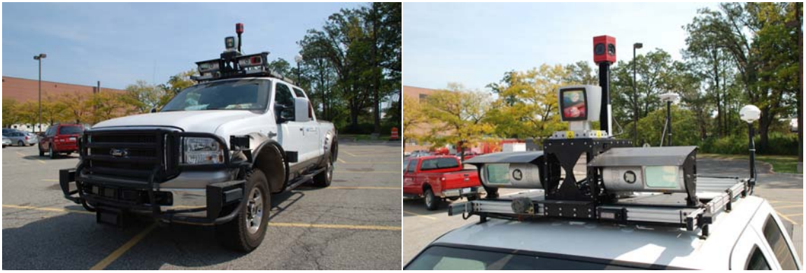
Figure 3.11 The modified Ford F-250 pickup truck with sensor configuration as described in appendix C. The 3D laser scanner [165] and the omnidirectional camera [82] are mounted on the roof of the vehicle.
