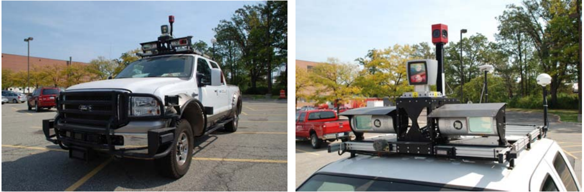
(a) Test vehicle mounted with 3D laser scanner and omnidirectional camera system
