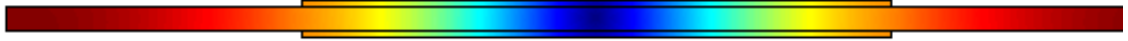
Figure 4.3: COMSOL Multiphysics simulation showing the total displacement of a parallel plate electrode contour mode resonator. Red indicates a large displacement and blue indicated a small displacement.
