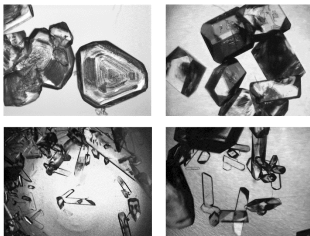
Figure 4.7. Morphology of acetaminophen crystals grown in the presence of p -acetamidostyrene. Clockwise from top left: no additive, 1 mM additive, 3 mM additive, and 6 mM additive.
