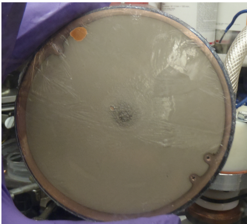
Figure 4.32: Example of electro-deposited lithium anode coverage from the potential hold anode. The deposition parameters are \sim 100 rpm wafer rotation, -1750 mV voltage vs \text{Li}/\text{Li}^+ , 400 C deposition cutoff. The outer copper ring is due to lack of line-of-sight to the lithium source wedge. The central buildup of dendritic lithium is a result of small angular velocity when near the axis of rotation.
