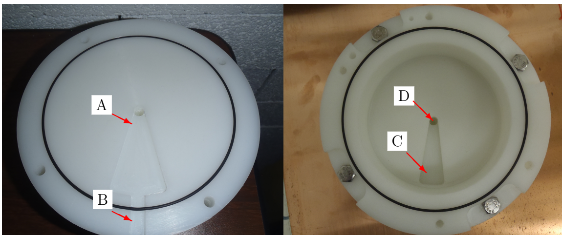
Figure 3.6: Left: Bottom of the lithium deposition chamber A) 30° radial section where lithium metal sheet resides, B) Lithium metal extending from the radial section sits in this channel. The extension protrudes from the edge of the chamber by \sim 1 cm, is folded back upon itself and a copper wire is sandwiched between. This fold is compressed by the top of the chamber to create a seal in conjunction with the Viton gasket. Right: Top of the lithium deposition chamber C) 20° radial section which masks the edges of the lithium sheet. D) Alignment hole for machining purposes. The hole during operation has a 1/4" diameter HDPE rod with a slit which holds the tip of the lithium sheet masking the tip (not shown).
