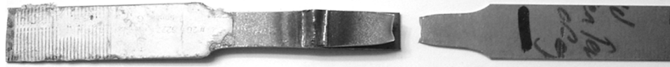
Figure 2.3. The failure location of an un-notched lap-shear specimen. The failure occurred in the base metal, away from the weld region.
