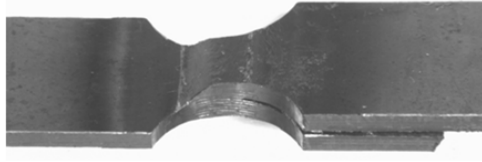
Figure 2.4. A close-up view near the weld of a notched lap-shear specimen.
