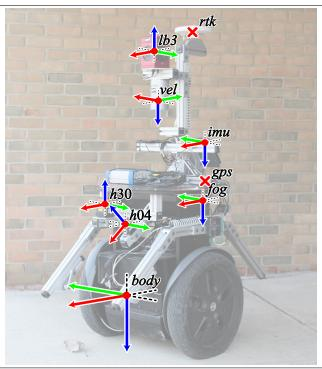
this body frame. An illustration of the body and sensor frames is provided in Fig. A.5. The 6-DOF transformations for each sensor, relative to the body frame, are given in Table A.2.
