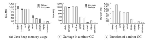
Figure 4.5: Java heap usage and GC behavior of sample workloads from SPECjvm2008 running in a 2GB VM; see Table 4.1 for workload descriptions. The Young generation of the Java heap is allowed to use at most 1GB memory.
