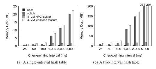
Figure 2.5: The memory cost of similarity compression using 256 byte chunks.
