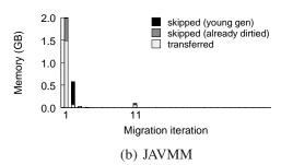
Figure 4.9: Amount of memory processed when migrating a VM running the compiler workload from SPECjvm2008. In (b), the 4–10th iterations of JAVMM each process less than 2MB of dirty memory.
