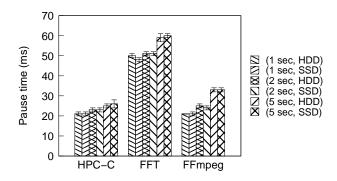
Figure 3.2: The VM pause time incurred for taking an incremental checkpoint. The legend is given in (configured checkpointing interval, fail-over image storage type).
