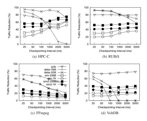
Figure 2.2: The traffic reductions achieved for a single protected VM running different workloads. The "sim-\*" lines show the traffic reductions achieved by similarity compression using different chunk sizes and a single-interval hash table, and the "sim2-\*" lines show those achieved using a two-interval hash table.
