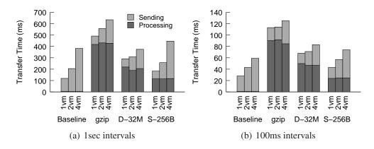
Figure 2.10: The breakdown of the checkpoint transfer times of a HPC-C VM measured in our HPC clusters consisting of 1, 2 and 4 VMs.
