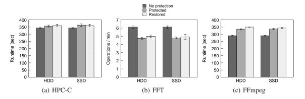
Figure 3.5: The performance of the workloads under different conditions: *no protection* and not checkpointed, *protected* and configured to be checkpointed every second, and *restored* from a failure that occurs halfway through the workload executions.
