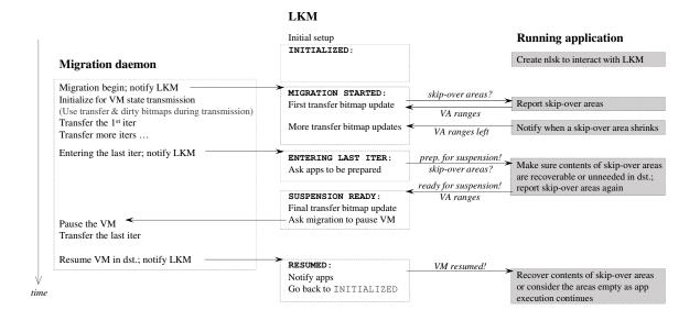
Figure 4.4: The workflow of application-assisted live migration.
