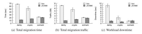
Figure 4.10: Performance of JAVMM and Xen live migration for workloads with different characteristics of Java heap usage.
