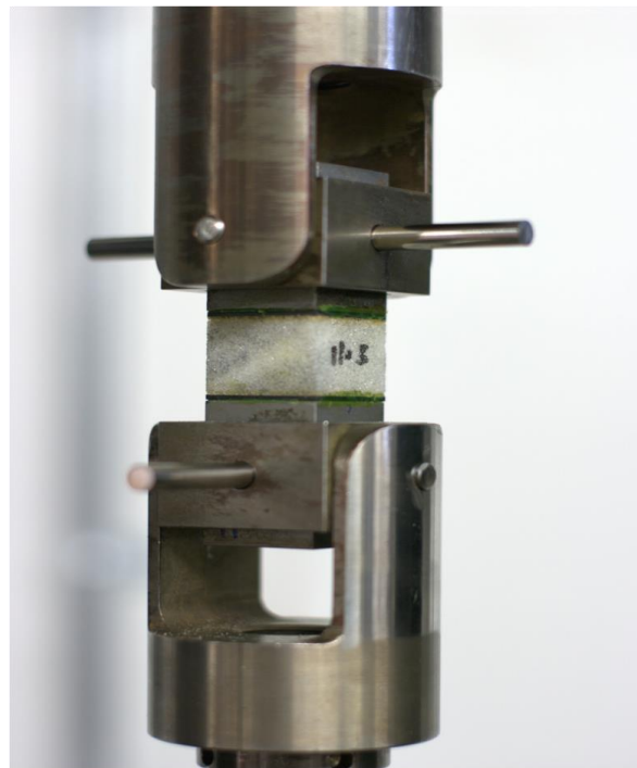
Figure 5.7: Flatwise tension specimen in experimental setup. (Image used with the permission of The Aerospace Corporation.)
