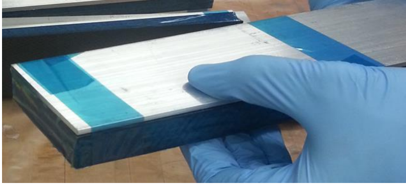
Figure 3.15. Image from BDCB fabrication showing taping of 3DFRFC edges. (Not to scale.)
