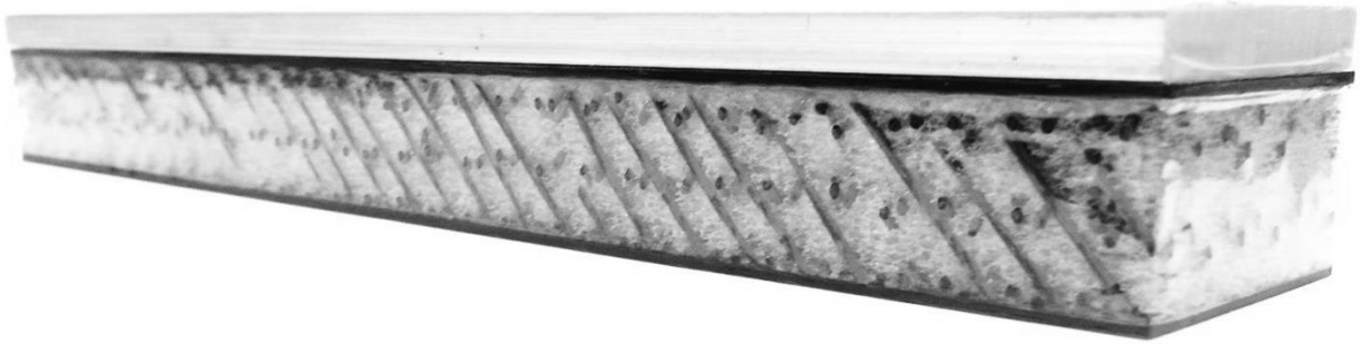
Figure 3.10. Fracture sample for measuring 3DFRFC properties. (Not to scale.)
