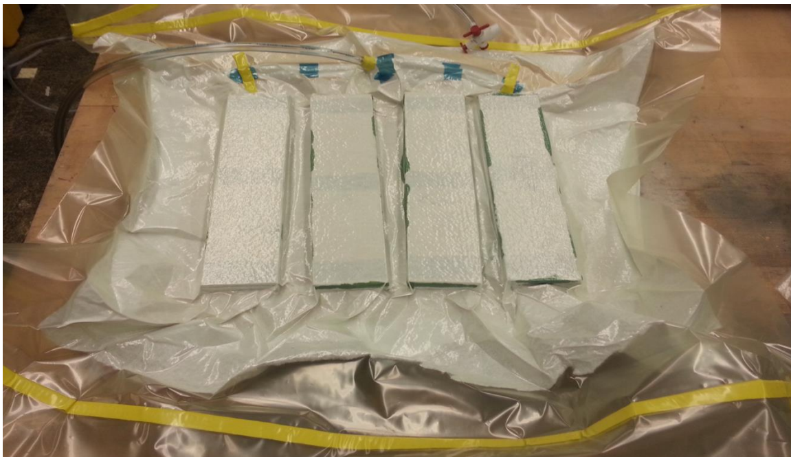
Figure 3.16. Vacuum bagged BDCB specimens.
