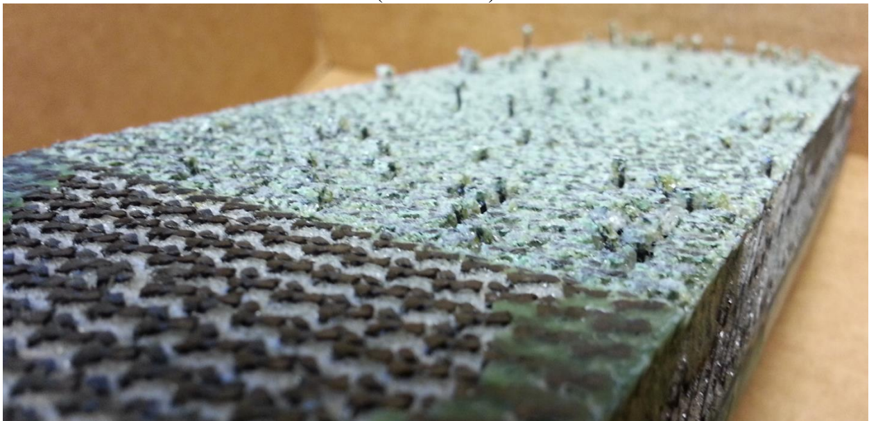
Figure 3.21. BDCB fracture surface (core side) showing higher percentage of partial pin pullout. (Not to scale.)
