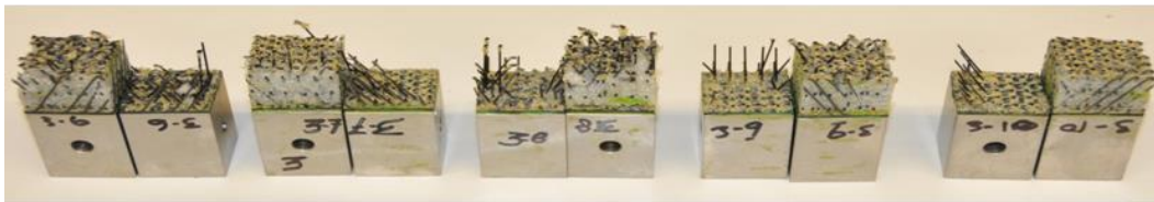
Figure 6.8. Failed cold temperature Size 1 3DFRFC FWT specimens. (Not to scale. Image used with the permission of The Aerospace Corporation.)
