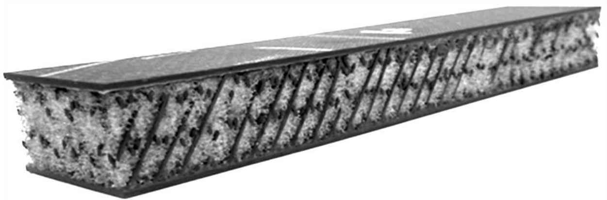
Figure 2.1. Sandwich composite made with a 3D fiber reinforced foam core. (Not to scale.)
