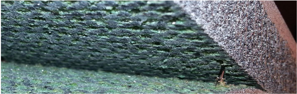
Figure 3.20. BDCB fracture surface showing pin pulling out during test. (Not to scale.)
