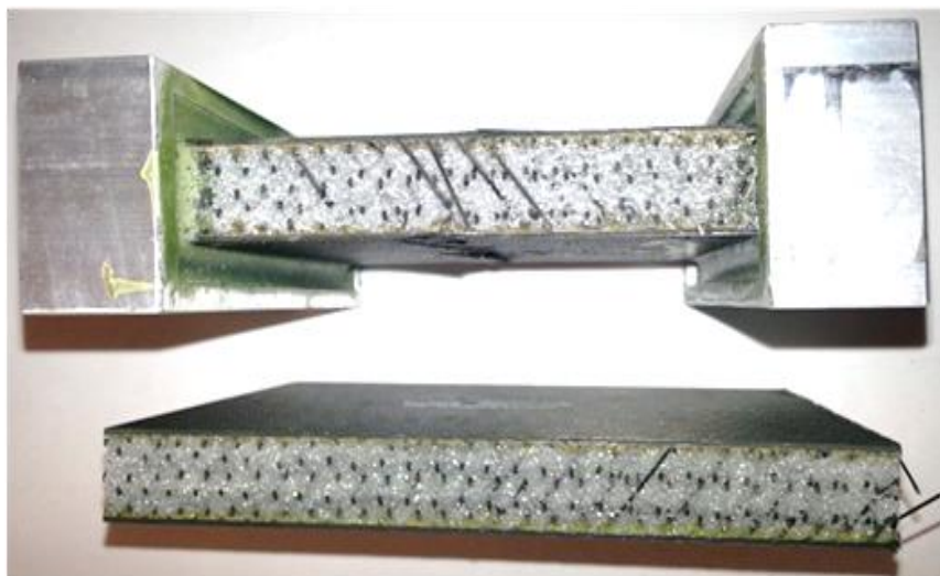
Figure 4.6. Edgewise Compression sample with potted ends (top) and with end failure (bottom). (Not to scale.)
