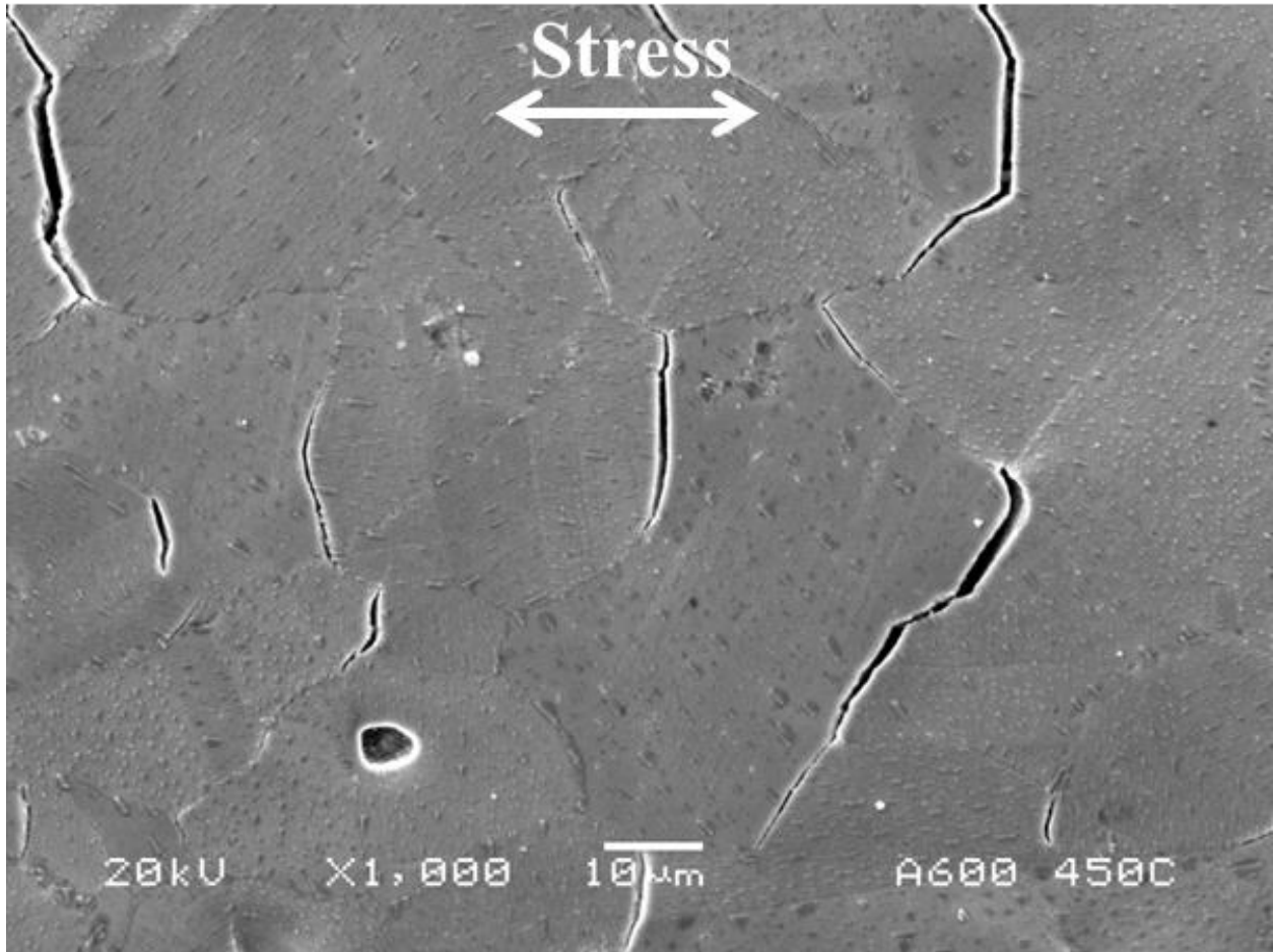
Figure 3.10. Gauge surface of Alloy 600 strained at 450°C in CERT to 8% at 3 \times 10^{-7} \text{ s}^{-1} showing cracking saturation.
