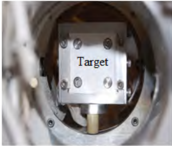
Figure 3.11: Electromagnet as a structural member to hold the target.
