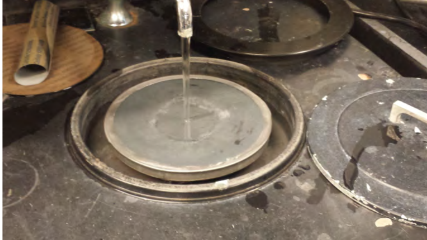
Figure 3.16: Polishing materials before tests on a grinding wheel using continuous supply of water.
