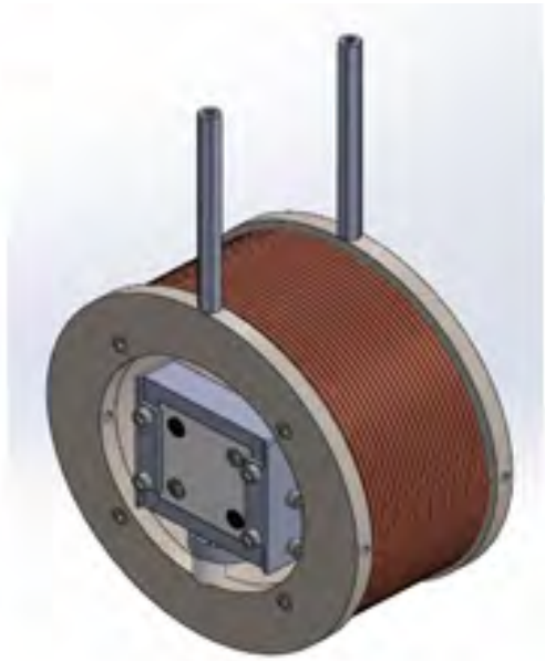
Figure 3.11: Electromagnet as a structural member to hold the target.
