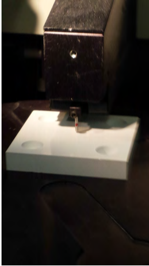
Figure 3.18: Measurement of surface roughness of HP grade BN performed using a stylus profilometer
