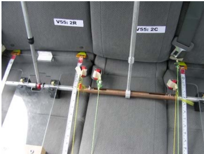
Figure 10. 2011 Honda Civic has the center webbing outboard of the left buckle (WAABbBwAAW)
