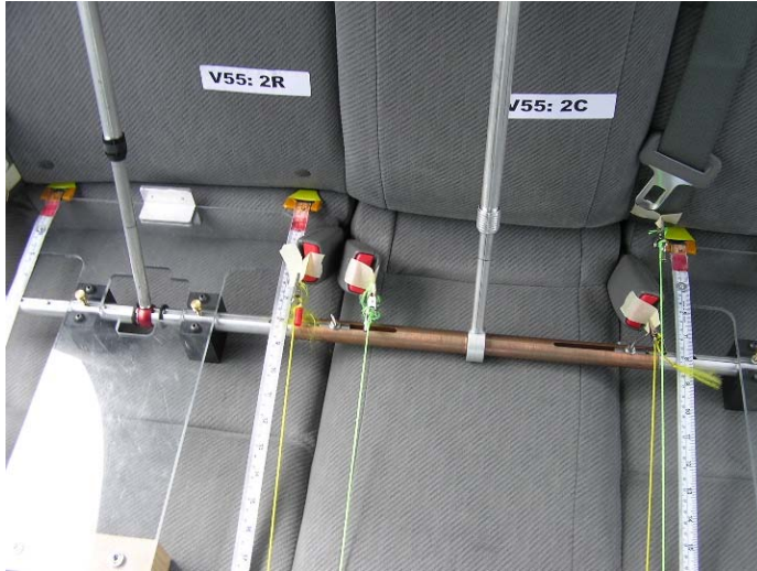
Figure 2. Example of “preferred” anchorage arrangement with lower anchors for the outboard positions placed in between the seat belt anchors for those positions.
