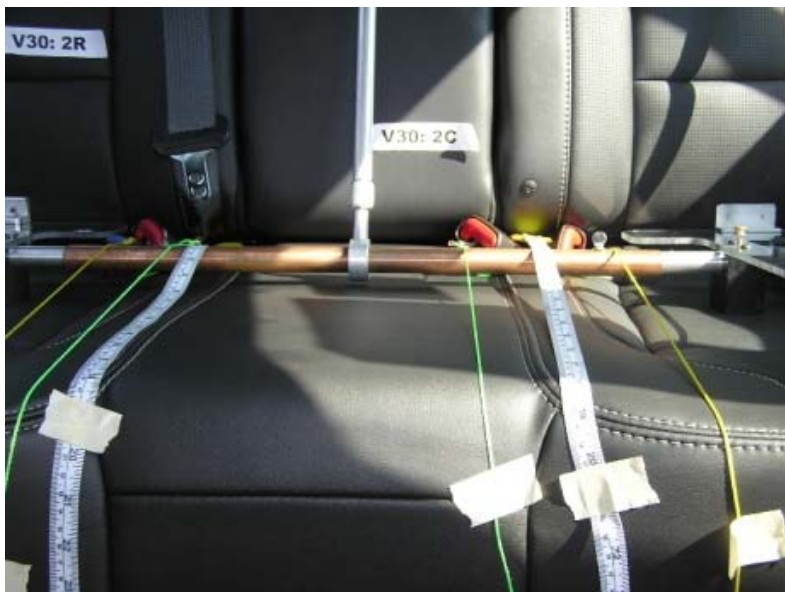
Figure 8. Arrangement of anchors in Ford Taurus, where the distance between the inboard lower anchors for the outboard positions is 280 mm.
