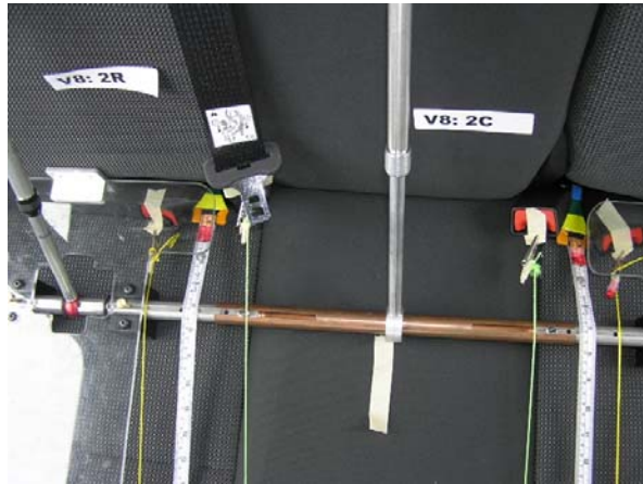
Figure 12. Lower anchor placement between center and outboard seat belt hardware would be conducive to improvised center LATCH.
