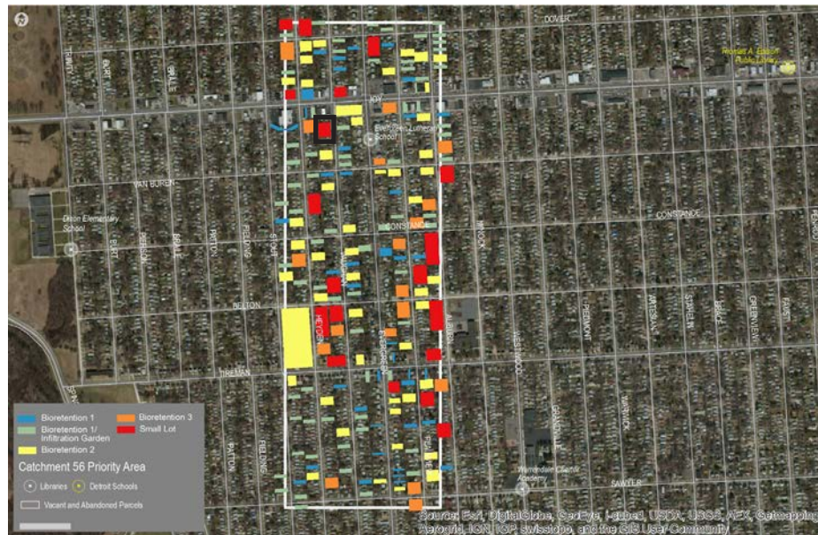
Figure IV-30: BMP Cluster Types in Priority Catchment Area 56
