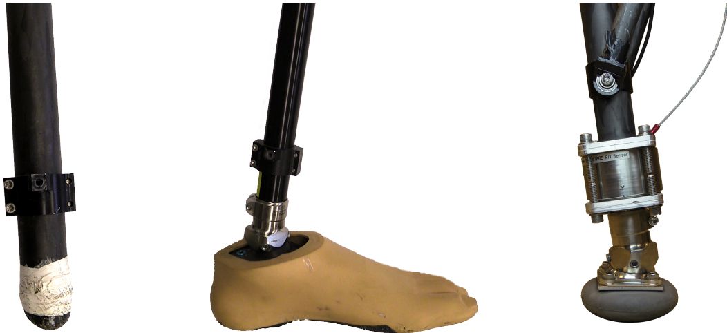
Figure 3.2: Different types of foot used on MARLO. From left to right: “point foot”, prosthetic foot, toroidal foot. Note the force/torque sensor mounted above the toroidal foot.
