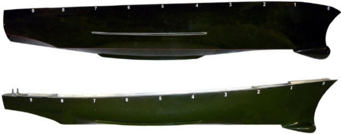
Figure 6.1: DTMB 5415 bare hull model from IIHR experiments. Top photograph shows the keel and both bilge keels
