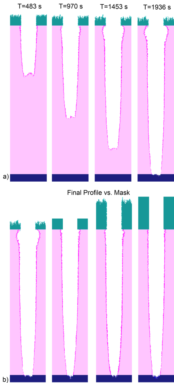
Fig. 7.12. Influence of profile with changing mask thickness and erosion for operating conditions ( \text{Ar}/\text{Cl}_2=80/20 , 20 mTorr, 200 sccm, 15 MHz coil power = 800 W and 600 V 15 MHz rf bias). a) Time sequential profiles of \text{Ar}/\text{Cl}_2 etching Si via with 60 nm thick mask considering mask erosion. b) 20% over etch profiles with 60 nm erosional mask, 60 nm hardmask, 180 nm erosional mask and 180 nm hardmask from left to right.
