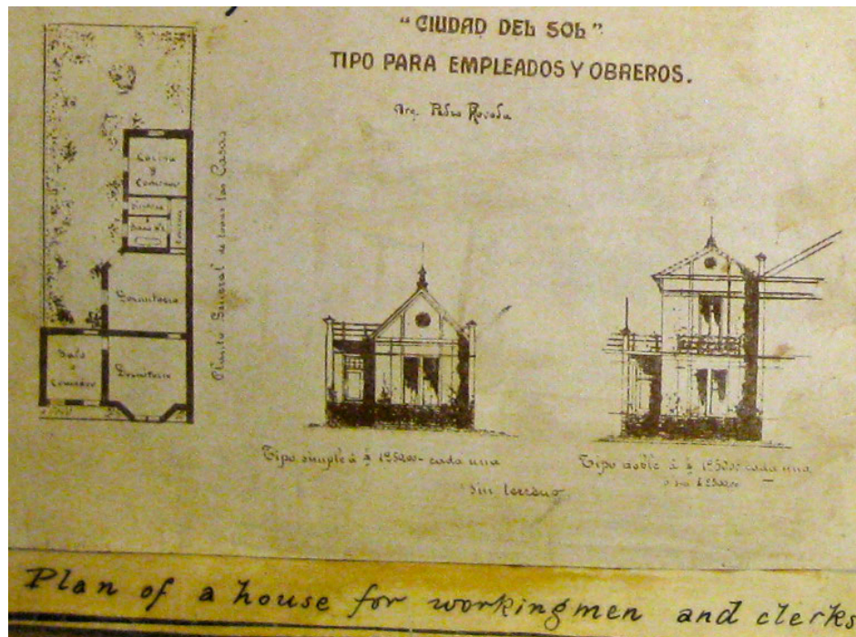
Figure 1:19 Roveda’s proposed four room (above) and five room (below) worker’s houses, plan and elevation drawings. The mixing of English and Spanish language in the drawings of this Italian designer suggests that he was reaching out to an international audience.
