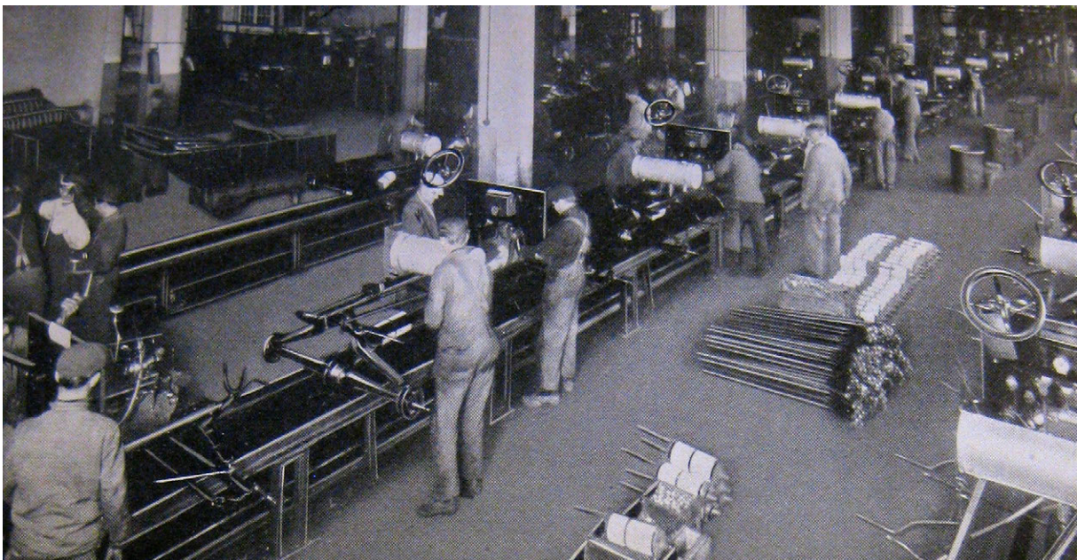
Figure I:2: The assembly line brings the chassis to the stationary worker in Ford's Highland Park Plant. Ford Motor Company, Ford Factory Facts (1915). Benson Ford Research Center.
