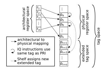
Figure 3.5: Extended tag space and mapping.
