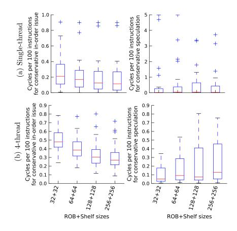
Figure 5.2: Potential stall cycles due to conservative mechanisms.
