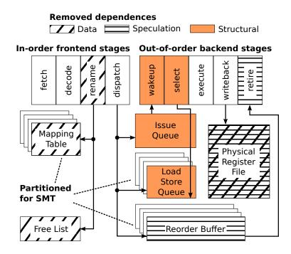
Figure 2.2: Baseline microarchitecture with SMT partitioning and OOO dependence removal.
