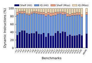
Figure 5.5: Steering hits/misses compared with ideal greedy algorithm.
