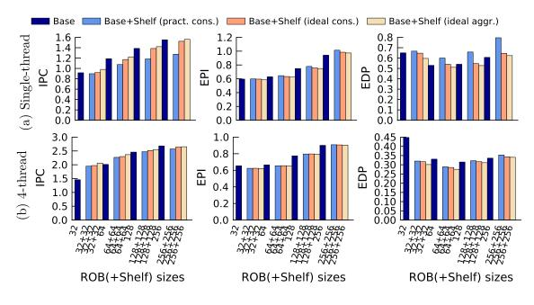
Figure 5.1: Comparison of doubling OOO structures against adding a shelf.
