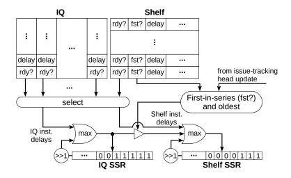
Figure 3.3: Delaying the shelf for speculation.
