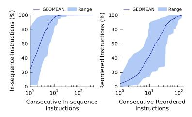
Figure 2.6: Weighted cumulative distribution of consecutive in-sequence and reordered instruction series lengths.
