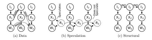
Figure 2.3: Removed dependences
