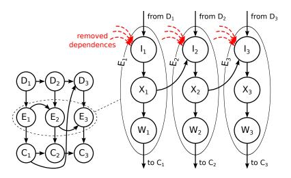
Figure 2.1: Dependence chain model for issue stage.
