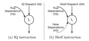
Figure 4.1: Issue stage dependences depending on steering.
