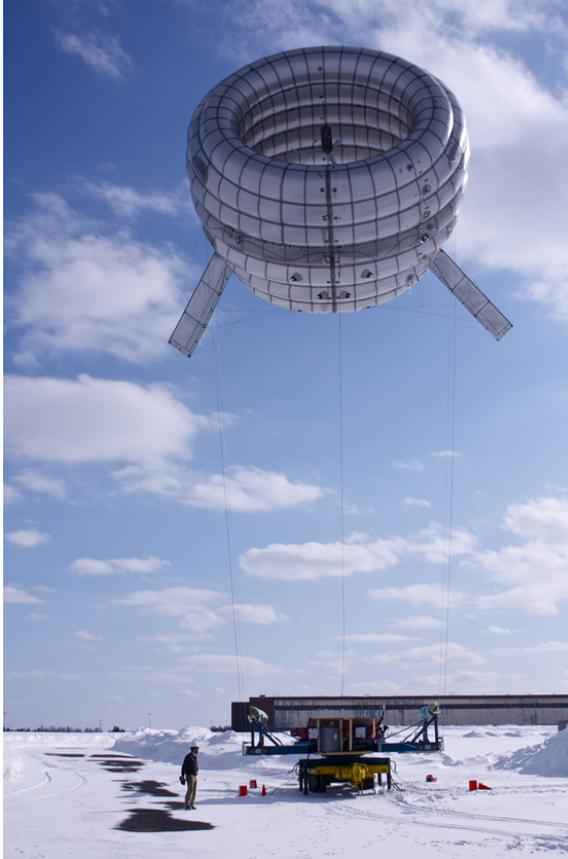
Figure 7.1: Photograph of Altaeros’s proof-of-concept system, which was flown at Loring Air Force Base during the winter of 2012 [46]
