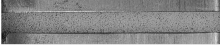
Figure 2.2: Side image showing the applied speckle and cropped raw image for compressive tests of the SC15
