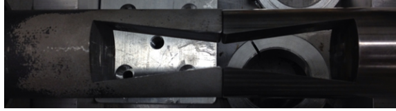
Figure 3.6: The ends of the bars after EDMing showing the profile
