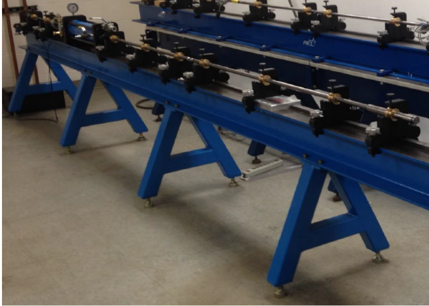
Figure 4.3: The Split Hopkinson Tensile Bar at the BLAST Lab (Photo courtesy of M. Pankow via REL)
