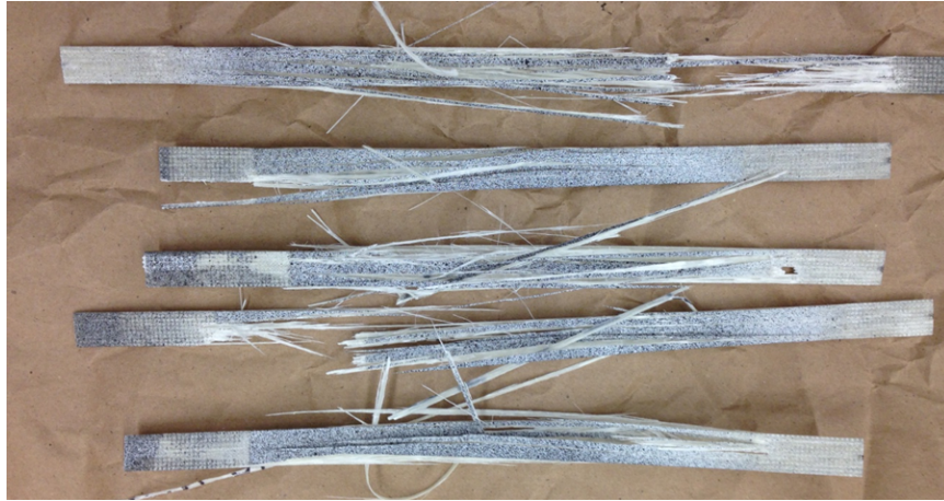
Figure 2.15: Photograph of experimentally tested unidirectional samples showing a high degree of fiber splitting
