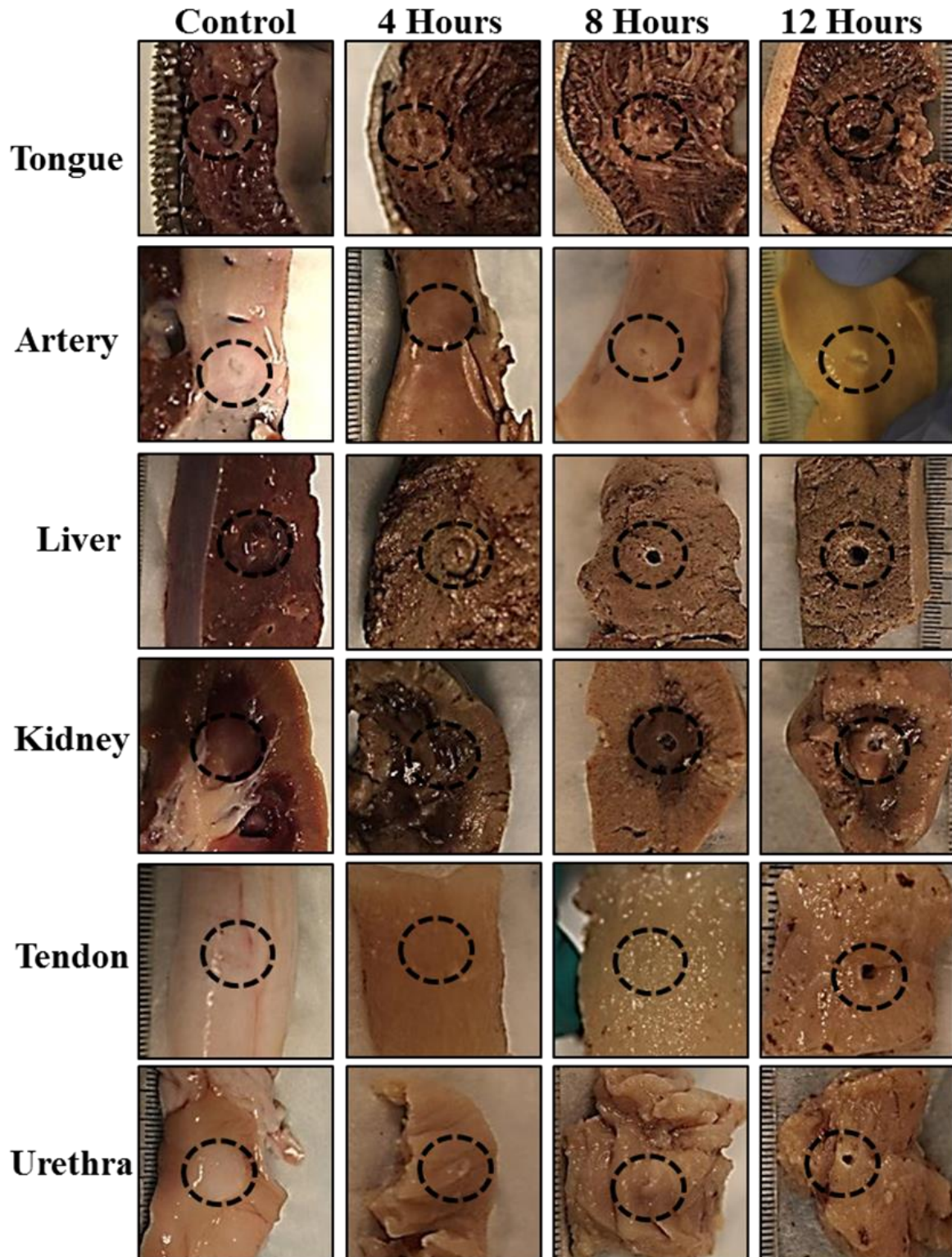
Figure 6.7. Morphological analysis of bovine tissues after histotripsy show tongue, artery, liver, kidney, and urethra were less susceptible to histotripsy after heating at 90°C for 4 hours while tendon was more susceptible to histotripsy after heating. All tissues became more susceptible to histotripsy after heating was continued for 8 and 12 hours (compared to 4 hour samples).
