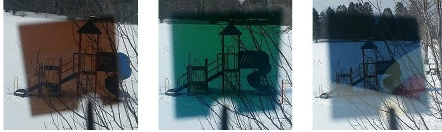
Figure 3.3.4 Optical photographs of fabricated visible wavelength filter devices on 2 cm x 2 cm glass.
