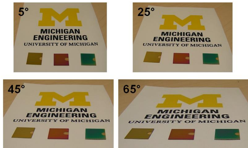
Figure 3.2.12 Photographs of the fabricated color filter devices taken from 5^\circ to 65^\circ . It is obvious that an original color can preserve even at very large angle ( 65^\circ ), confirming the angle invariant characteristic of the proposed filters.
