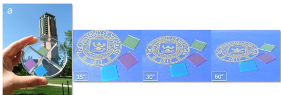
Figure 6.2.4 Images of the fabricated devices displaying vivid cyan, magenta, and yellow (CMY) colors. The colored cells clearly demonstrate angle-insensitive performance at large angles of incidence (15°, 30°, and 60°).
