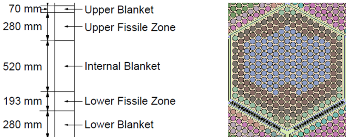
Figure B.8: RBWR-type assembly axial view (left) and radial view (right)
