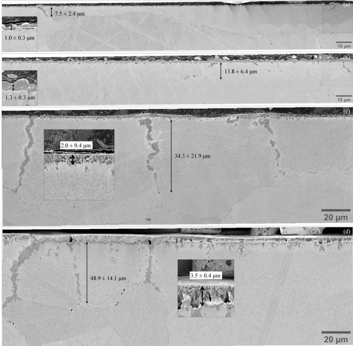
Figure 4-5 SEM images comparing the surface damage in Alloy 617 crept at 800°C in different environments and loading types. The images show the effect on the surface scale thickness and depth of intrusions of the different stress/strain/total test time conditions: (a) 50 MPa/1.9%/211 h, (b) 10/50 MPa/2.3%/690 h, (c) 50 MPa/1.7%/206 h, and (d) 10/50 MPa/2.1%/553 h. The studies were conducted in He- \leq 0.1 ppm O 2 (a,b) and He-CO/CO 2 =1320 (c,d) environments. The stress axis is horizontal and in the plane of the page.
