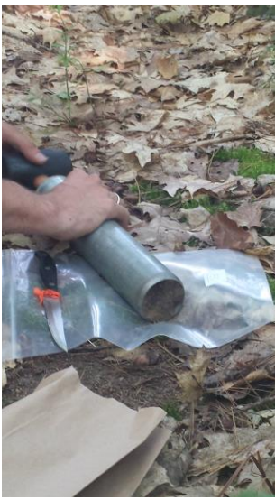
Fig 1: Soils samples being collected using the cylinder and mallet
