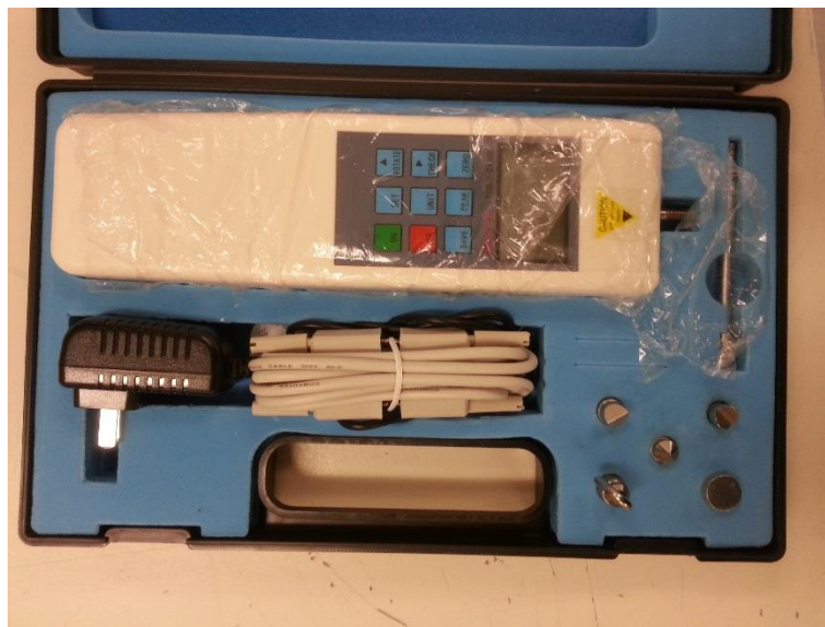
Figure G.4.2: Picture of Model HF-200 Digital Force Gauge used in the empirical testing of vacuum chucking system
