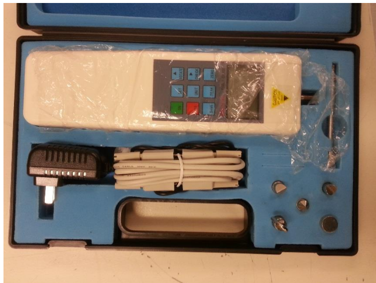
Figure G.9.7: Picture of Model HF-200 Digital Force Gauge used in the empirical testing of vacuum chucking system
