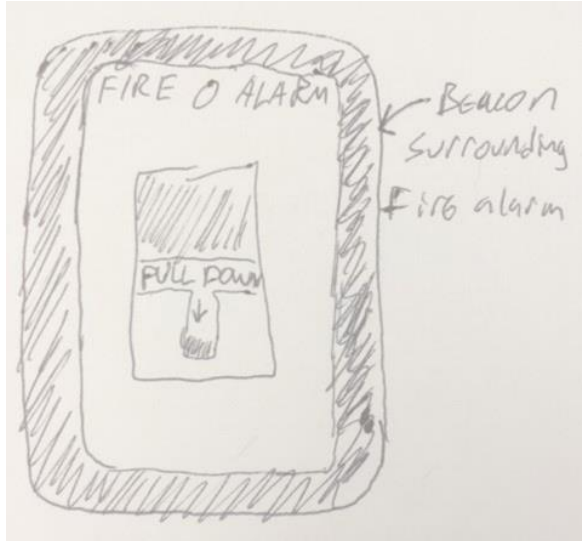
Figure 4: Beacon integrated into fire alarm
