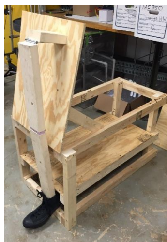
Figure 4: The wooden frame dimensioned from Ben's wheelchair.
