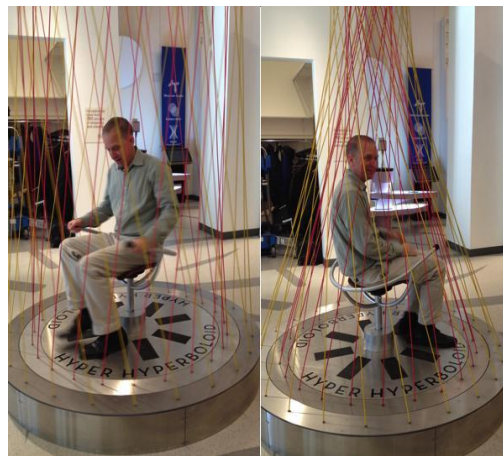
Figure 2: Elastic cords show how surface of hyperboloid of revolution changes as angle of straight lines changes. [3]
