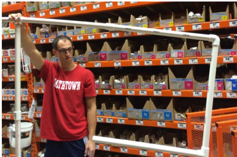
Figure 35: Mockup Construction Shows Sagging Corner of Frame
