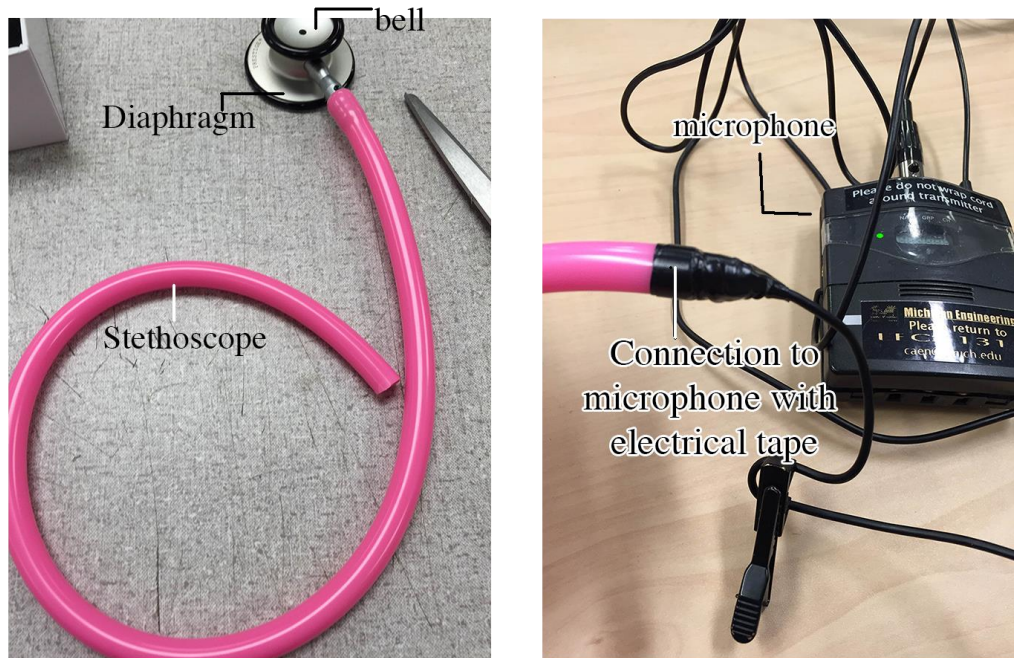
Figure 33: Set up for the microphone stethoscope. Left- cut stethoscope. Right - Connection to microphone
