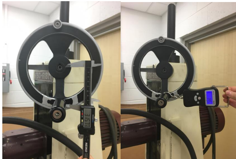
Figure 12. Experimental Setup for Torque Measurement of Z-Axis (Left for lever arm measurement, Right for force measurement)
