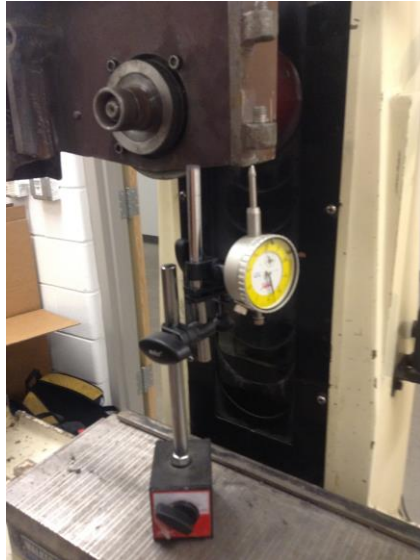
Figure 13. The height gauge test setup used to verify the y and z axes.
