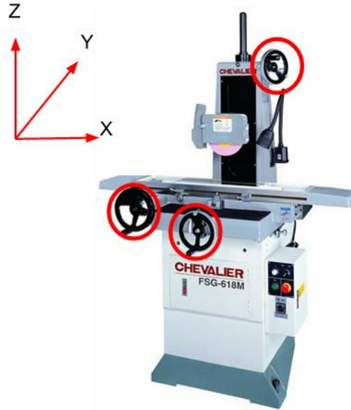
Figure 1. Chevalier FSG-618M surface grinder the team has been tasked with adding automation to. Axes are defined as in this figure, with X being the longitudinal axis of table travel.
