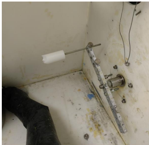
Figure A.2: A CCSD valve mold attached to the rotisserie.
