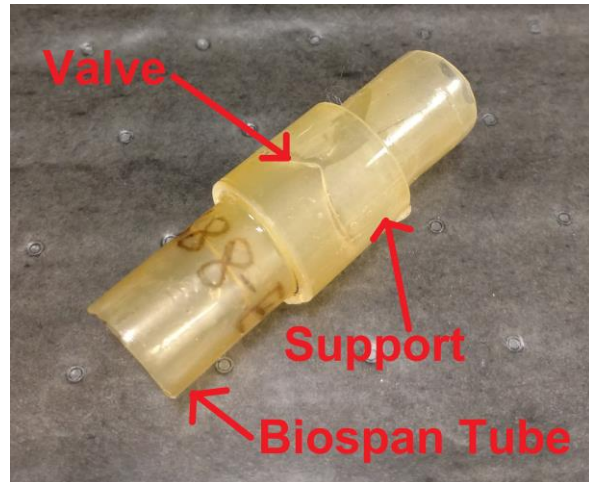
Figure A.5: A valve glued into a biospan tube with a rigid support tube.
