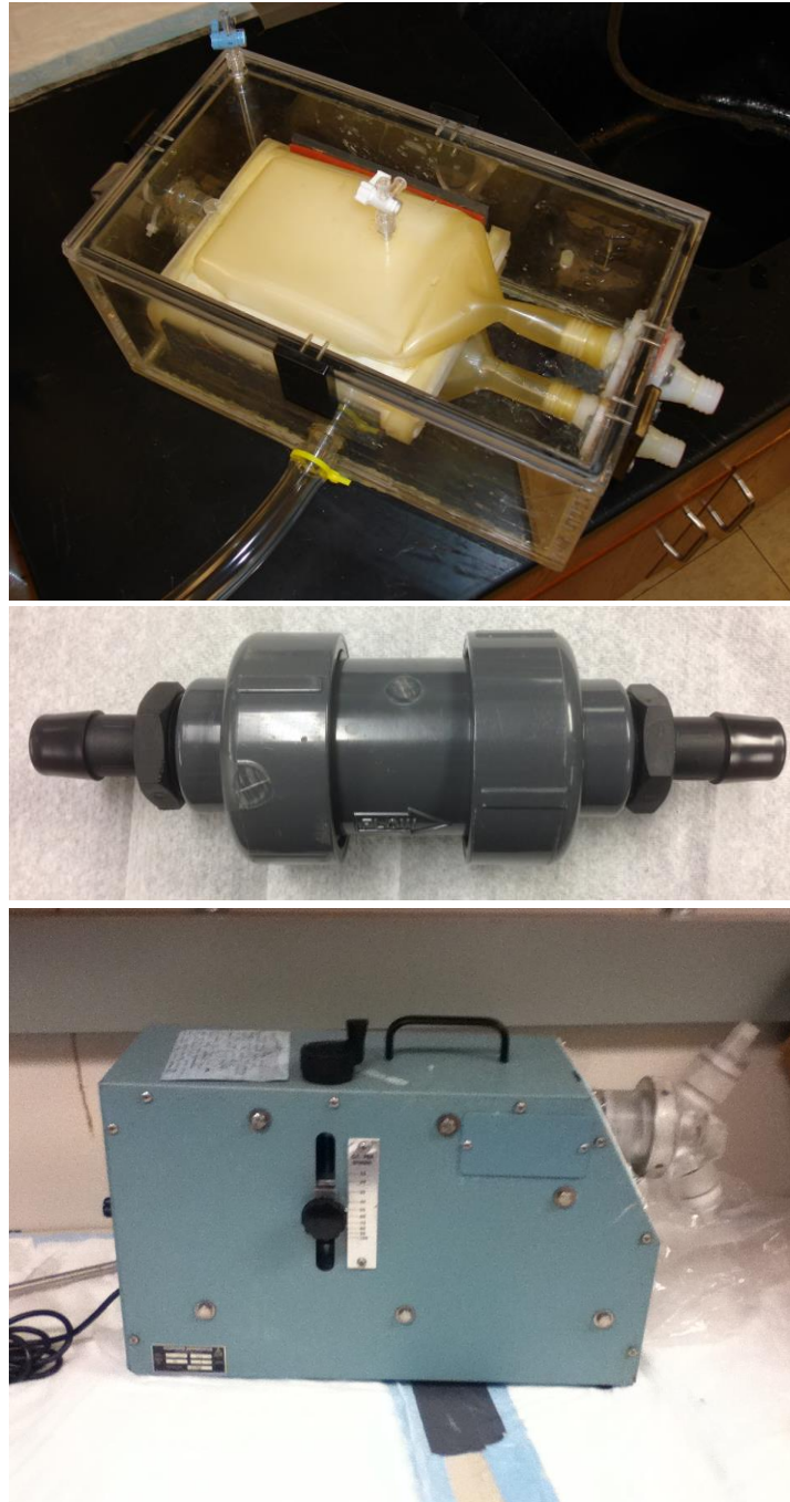
Figure 2.2: Top: The original prototype CCSD enclosure and gas exchanger assembly. Middle: The original prototype CCSD external ball valves. Bottom: The original prototype CCSD Harvard pulsatile pump.
