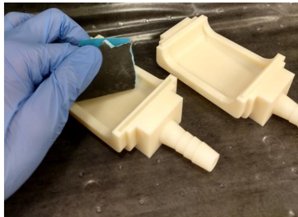
Figure B.3: Sanding of the inside surfaces of the PAD housing.
