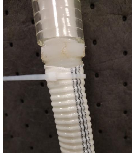
Figure C.3: An extension connector threaded onto a synthetic graft.
