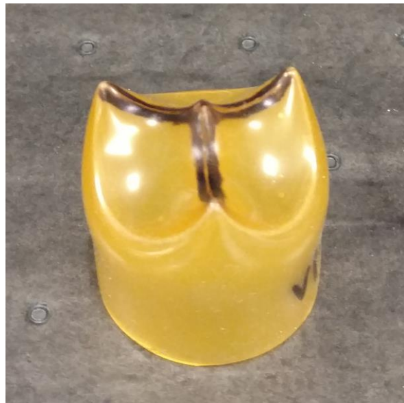
Figure A.4: A cut to length CCSD valve with colored leaflet edges.
