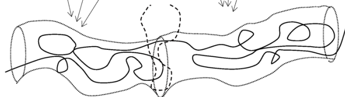
Figure 3.1. Schematic step-wise representation of tube enlargement mechanism during fast elongational flows: (a) No flow conditions; equilibrium random walk, (b) Tube orientation, backfolding and stretch due to fast flows, (c) Loss of entanglements, merging of tube segments and tube diameter enlargement.
