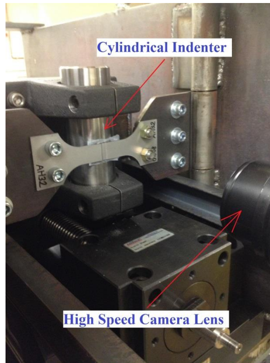
Figure 4-4 Set-up for cylindrical indenter experiments: The diameter of the cylindrical indenter is 2 inches (equivalent to 50.8 mm) and the test specimen depicted is an 18mm-width specimen with a 4 mm groove.
