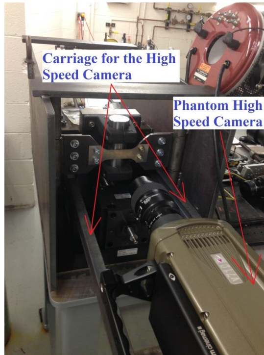
Figure 4-5 The indenter set-up with camera carriage: The carriage is attached to the cylindrical indenter support system so the camera moves with the indenter and thus enables video to be captured at a constant distance from the test sample in contact with the indenter surface (Courtesy of Prof. Marc Perlin).
