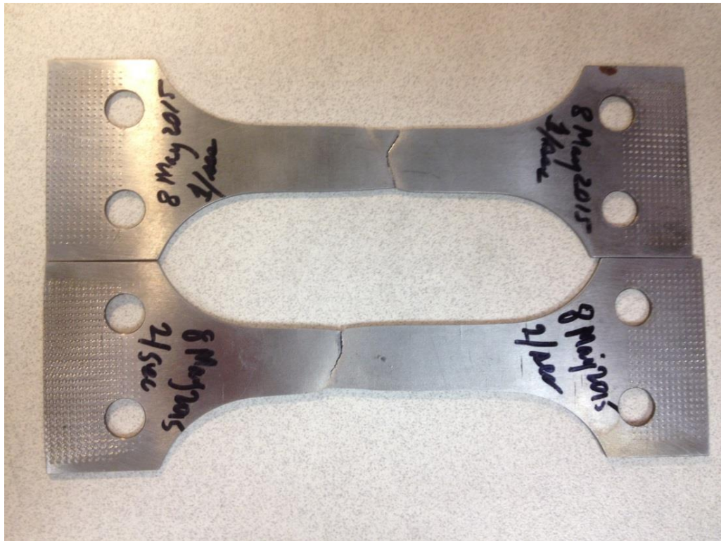
Figure 4-10 Fractured specimens of high speed tensile tests. The specimens used in the tests were 18mm-width specimens (without groove). The specimen on the top was subjected to strain rate of 1 \text{ s}^{-1} , while the one on the bottom was subjected to 2 \text{ s}^{-1} .
