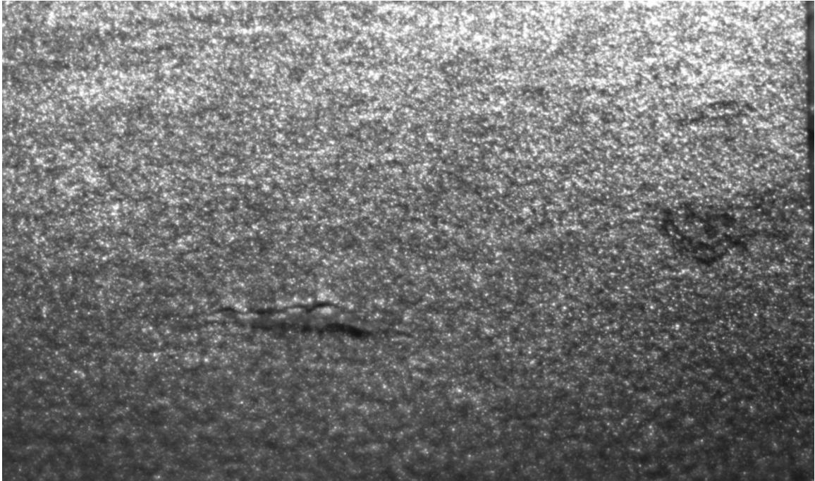
Figure 4-88 Nital etched AH32 steel 18mm-width-specimen without groove at Frame 24250; that is, a 49.276 mm indentation had been applied.
