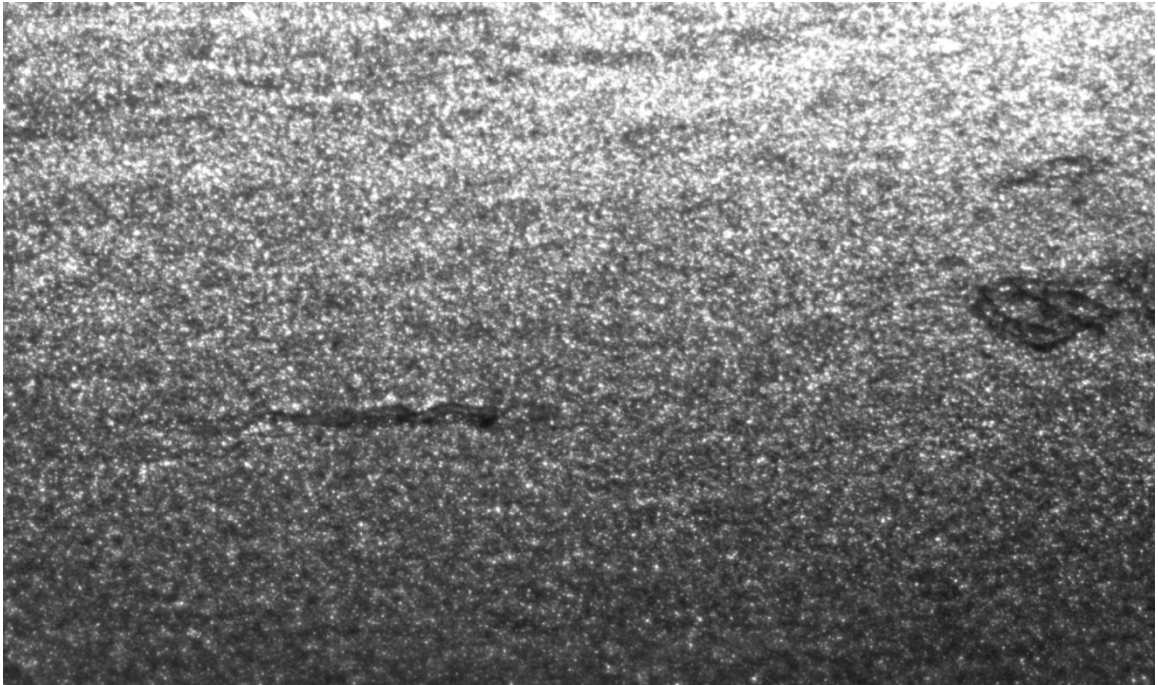
Figure 4-87 Nital etched AH32 steel 18mm-width-specimen without groove at Frame 22250; that is, a 45.212 mm indentation had been applied.
