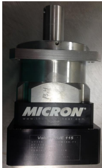
Figure 4-7 Micron VT115-005-0-RM100-71 10:1 ratio gear reducer.
