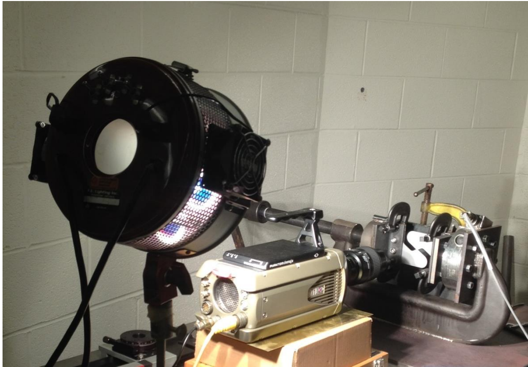
Figure 4-2 An example experimental set-up for a uniaxial test: The test specimen depicted is a shear specimen (without a groove). Note that the test specimen is adapted from Bao & Wierzbicki's (2004) specimen design for pure shear tests.
