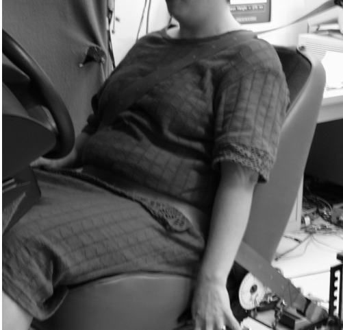
Figure 58a. Test session 2, shoulder belt 20°, lap belt 40°.
