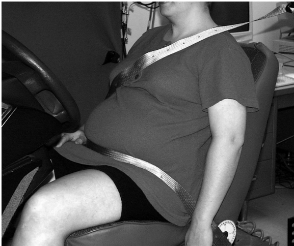
Figure 58c. Test session 3, shoulder belt 20°, lap belt 60°.
