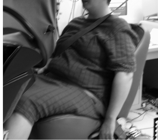
Figure 58b. Test session 2, shoulder belt 60°, lap belt 60°.
