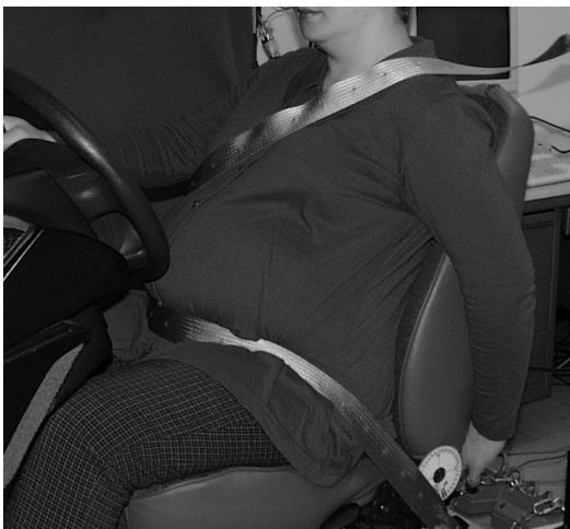
Figure 58e. Test session 4, shoulder belt 20°, lap belt 60°.
