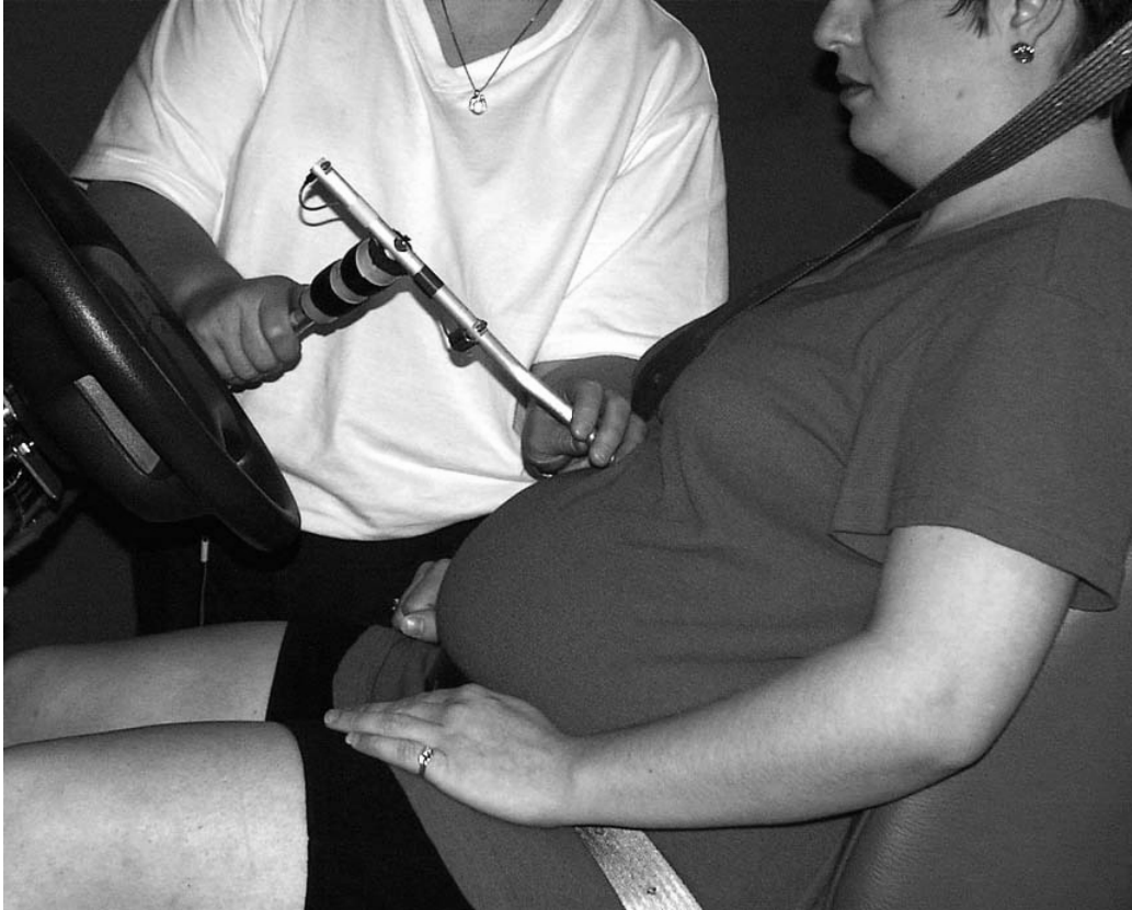
Figure 7. Measurement of abdomen contour with sonic-digitizer probe.
