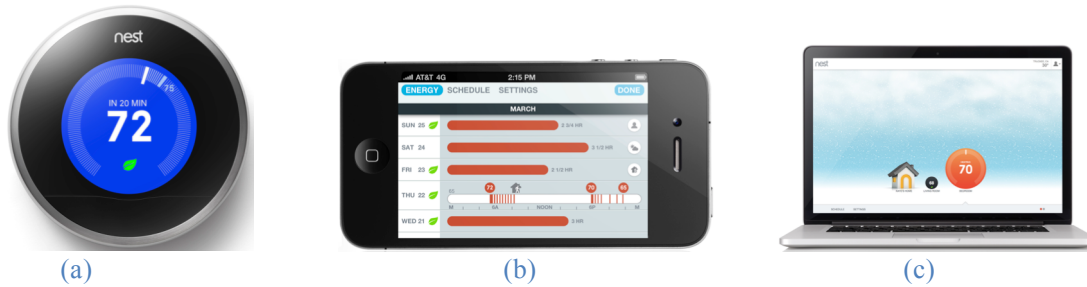
Figure 6. Users can control the Nest via the wall-mounted display (a), a mobile app (b), or a web app (c). © Nest Labs
