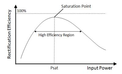
Figure 1.5. Typical rectification efficiency vs. input power of a P/N diode
