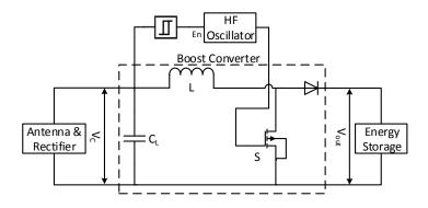
Figure 3.9. Topology of the power management unit, with dashed box showing the boost converter.
