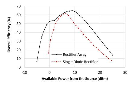
Figure 4.21. The measured overall efficiency (considering both the rectification loss and impedance mismatch reflection) for the wide dynamic range rectifier array, in comparison to a single diode rectifier circuit optimized for the highest efficiency.
