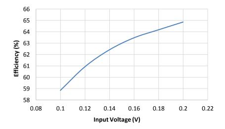
Figure 3.10. Measured efficiency of the boost converter versus input voltage
