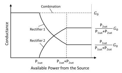
Figure 4.4. The ideal conductance variation curves of Rectifier 1, Rectifier 2, and their combination.
