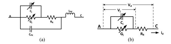
Figure 3.5. (a) Full nonlinear model and (b) de-embedded model for a PIN junction diode
