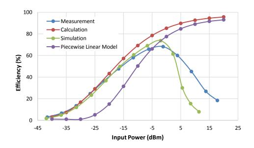
Figure 3.7. Rectification efficiency versus input power at 900 MHz for  $R_L = 3 k\Omega$ . Results generated from the proposed analysis, the conventional piecewise linear analysis, ADS Harmonic simulation, and experiment were plotted against various input power.
