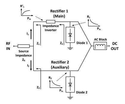
Figure 4.11. Operation principle of the adaptive power distribution rectifier array: source impedance modulation perspective.
