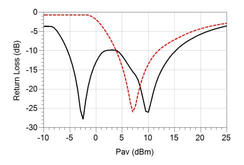
Figure 4.16. Simulated return loss for the adaptive power distribution circuit, in comparison with the return loss for a single diode rectifier circuit designed with the same device and optimized at the same frequency. Black solid curve shows the return loss of the adaptive power distribution circuit, while the red dashed curve shows the return loss of the single diode rectifier circuit.
