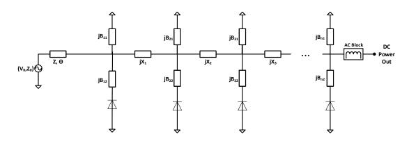
Figure 4.8. An example realization of the multi-way power distribution rectifier circuit scheme (based on lumped-elements).
