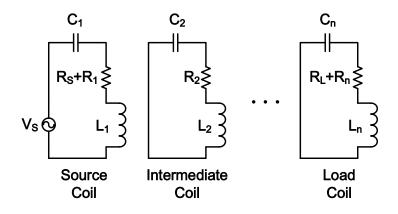
Figure 1.3. Equivalent circuit of a WPT system with multiple resonant coils.
