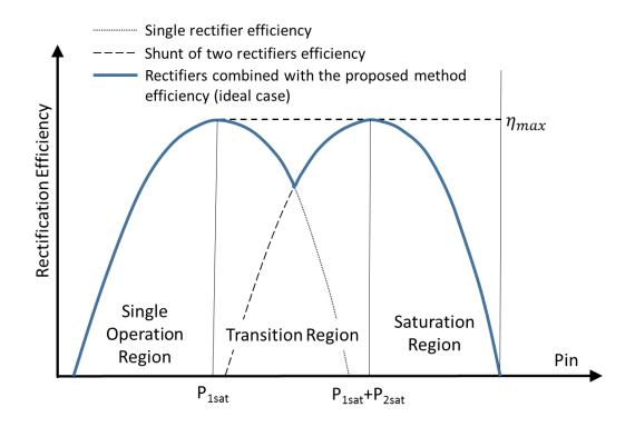
Figure 4.6. The comparison of rectification efficiencies: one single rectifiers; simple shunt of two rectifiers; and adaptive power distribution rectifier array circuit described in this dissertation.
