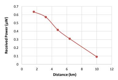
Figure 3.16. Received power versus distance to a local AM broadcasting station (WXYT)
