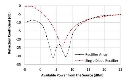
Figure 4.20. The measured reflection coefficient for the wide dynamic range rectifier array, in comparison to a single diode rectifier circuit optimized at the same frequency.
