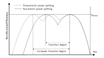
Figure 4.9. Multi-device (shown with the example of three-way rectifier array) power split efficiency, in comparison with a two-device rectifier array.
