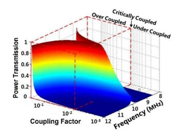
Figure 1.4. Transfer efficiency vs operation frequency and coupling factor; showing the frequency splitting phenomenon.
