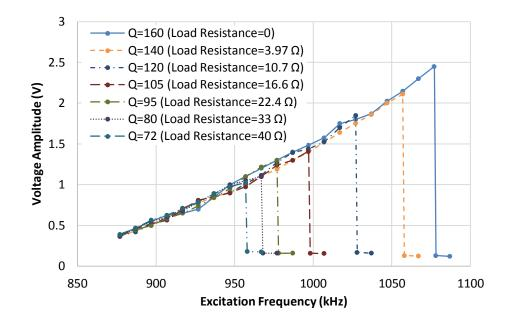
Figure 2.17. Measured voltage amplitude as functions of excitation frequencies with different loaded Q values.
