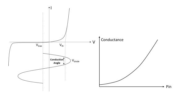
Figure 4.2. Conduction angle of diode and conductance vs. input power level (parasitic reactive components are cancelled with impedance transformation network)
