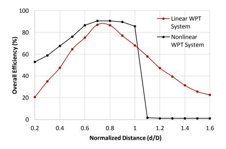
Figure 2.21. Measured transfer efficiencies (defined as  $\eta = P_{out}/P_{av}$ ) of both the nonlinear WPT circuit and the conventional linear WPT circuit as a function of normalized coupling distance to the coil diameter (d/D).
