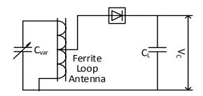
Figure 3.3. Configuration of the antenna and rectifier circuit
