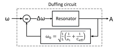
Figure 2.5. Negative feedback process in a Duffing resonator circuit, showing the feedback term provided by the nonlinear capacitor.
