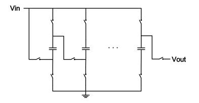
Figure 1.8. An example of switched capacitor voltage converter circuit.
