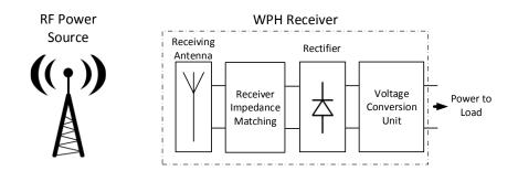
Figure 1.6. Block diagram of a typical WPH system
