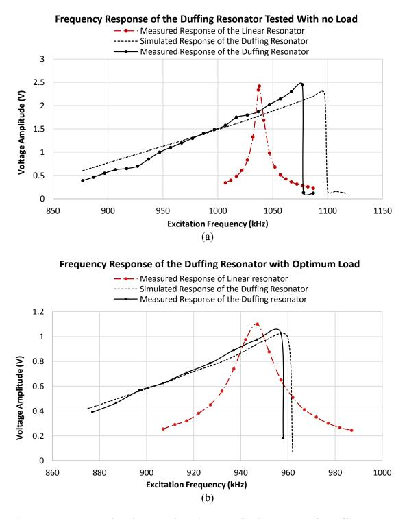
Figure 3.20. Comparison between the voltage amplitude response of a Duffing resonator based EM harvester and a linear resonator based EM harvester. (a) The simulation and measurement results for the Duffing resonator in comparison with the linear resonator without a load, and (b) the simulation and measurement results for the Duffing resonator in comparison with the linear resonator, when both circuits are connected to matched loads ( $R_L = R_S = 33 \Omega$ ).
