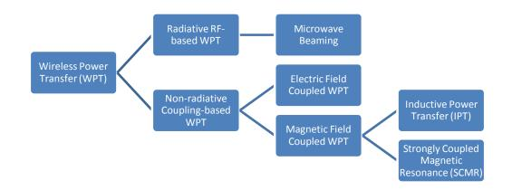
Figure 1.1. Summary of different wireless power transfer technologies
