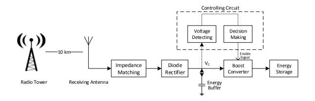
Figure 3.1. Block diagram of the medium wave wireless power harvester
