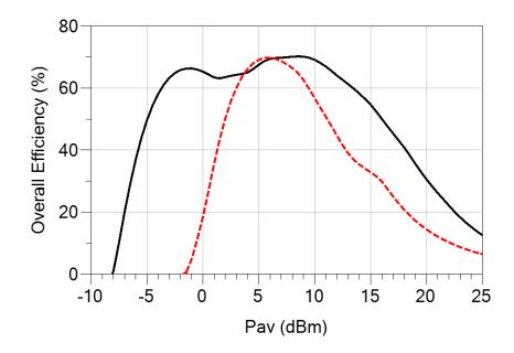
Figure 4.17. Simulated overall efficiency for the adaptive power distribution circuit, in comparison with the return loss for a single diode rectifier circuit designed with the same device and optimized at the same frequency. Black solid curve shows the overall efficiency of the adaptive power distribution circuit, while the red dashed curve shows the overall efficiency of the single diode rectifier circuit.
