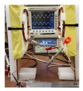
Figure 2.20. Photograph of the two-coil WPT system employing a Duffing resonator
