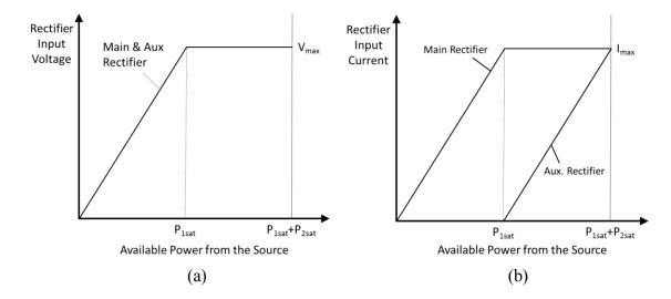
Figure 4.12. Adaptive power distribution rectifier array operation principles: (a) device voltages; and (b) device currents at different available power levels. Pictures show the case of even power splitting with ideal devices.
