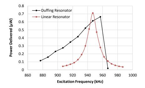
Figure 3.21. Measured output power of a Duffing resonator in comparison with a linear LC resonator. Both circuits are optimally loaded (equivalent load resistance matches to  $R_s$ ). Power available from the source is 0.7  $\mu$ W for both cases.
