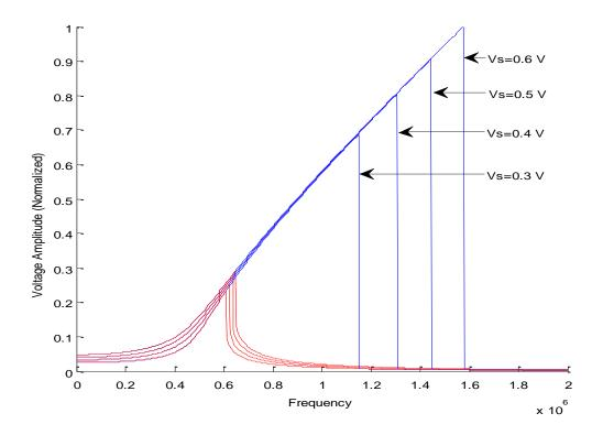
Figure 2.10. The frequency response of the Duffing resonator circuit for different excitation amplitudes (Vs) from 0.3 V to 0.6 V. The solid blue curve shows the high-amplitude equilibrium points at different frequencies, while the solid red curve shows all the low-amplitude equilibrium points.
