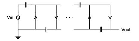
Figure 1.7. An example of voltage multiplier circuit.
