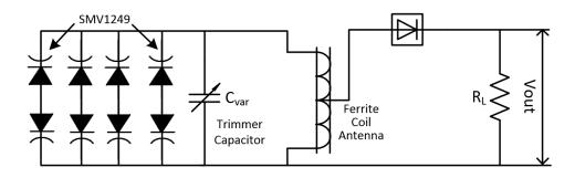
Figure 3.17. Circuit of the 1 MHz WPH receiver employing a Duffing resonator
