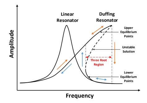
Figure 2.1. The amplitude-frequency response of a Duffing resonator circuit. Orange and blue arrows show the hysteresis loop and jump phenomenon.
