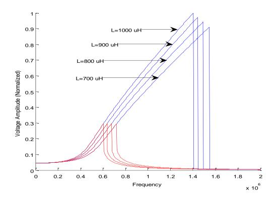
Figure 2.12. The frequency response of the Duffing resonator circuit for different inductance values ranging from 700  $\mu$ H to 1000  $\mu$ H. The solid blue curve shows the high-amplitude equilibrium points, while the solid red curve shows the low-amplitude equilibrium points.
