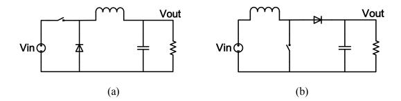
Figure 1.9. (a) Buck converter circuit; and (b) boost converter circuit.
