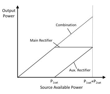
Figure 4.13. Adaptive power distribution rectifier array operation principles: output power at different available power levels. Pictures show the case of even power splitting with ideal devices.
