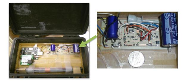
Figure 3.12. Photograph of the medium wave energy harvesting circuit.
