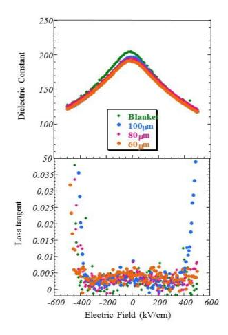
Figure 2.7. An example of BST varactors: measured dielectric tunability curve and loss tangent for BST varactors with different sizes [110]
