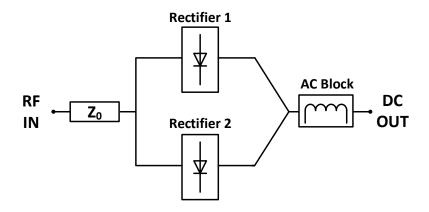
Figure 4.3. A basic block diagram intended to describe the operating principles of the adaptive power distribution rectifier array. The block diagram uses two individual rectifiers.
