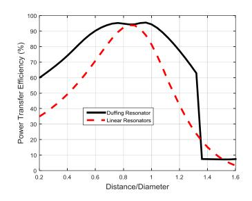
Figure 2.19. Simulated efficiency versus normalized distance (d/D) for the WPT circuit with nonlinear resonator in the secondary coil, in comparison with the efficiency for a WPT circuit with linear resonator of the same Q value.
