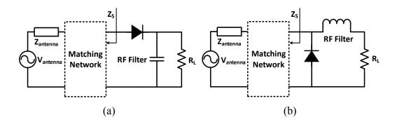
Figure 3.4. (a) Series and (b) shunt connected single diode rectifier
