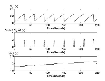
Figure 3.13. Waveform of  $V_c$  and  $V_{out}$  of the boost converter and the control signal given by the Schmitt trigger circuit. The reference voltages of the Schmitt trigger circuit,  $V_{high}$  and  $V_{low}$ , were set to 0.2 V and 0.08 V respectively.
