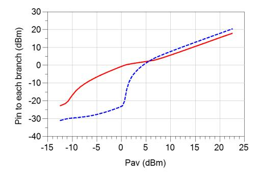
Figure 4.15. Simulated RF power distributed to each rectifier device as functions of available power level from the source. Red solid curve shows the RF power distributed to Rectifier 1, while the blue dashed curve shows the RF power distributed to Rectifier 2.
