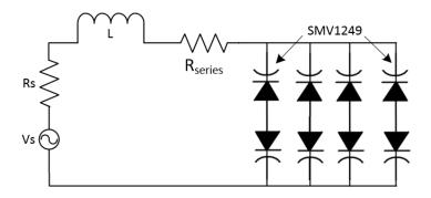
Figure 2.15. Diagram of the 1 MHz WPH system employing a Duffing resonator
