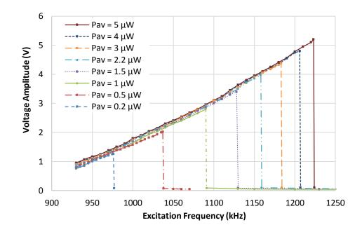
Figure 2.16. Measured voltage amplitude as functions of excitation frequencies at different available power levels from the source.
