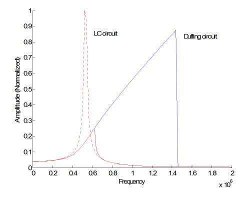
Figure 2.9. The frequency response of the Duffing resonator circuit, in comparison with a LC circuit with the same Q. For the Duffing resonator, the solid blue curve shows the high-amplitude equilibrium points at different frequencies, while the solid red curve shows the low-amplitude equilibrium points. The dashed red curve shows the amplitude response of the linear resonator used for comparison.
