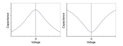
Figure 2.4. Symmetric C-V curves for nonlinear capacitors: (a) bell-shaped curve and (b) well-shaped curve.
