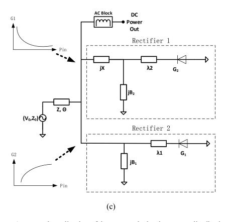
Figure 4.7. An example realization of the proposed adaptive power distribution rectifier circuit scheme: (a) lumped-element based design; (b) the rearranged form of the circuit and the input conductance versus power for each branch.
