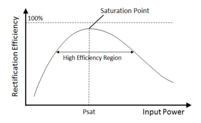
Figure 4.1. Typical rectification efficiency vs. input power of a P/N diode
