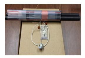
Figure 3.18. Photograph of the 1 MHz WPH circuit (excluding boost converter and control circuit) employing a Duffing resonator
