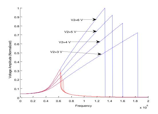
Figure 2.14. The frequency responses of the BST-based Duffing resonator circuits with different  $V_2$  values. The solid blue curve shows the high-amplitude equilibrium points, while the solid red curve shows the low-amplitude equilibrium points.
