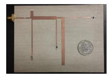
Figure 4.18. A photograph of the two-way wide dynamic range rectifier array.
