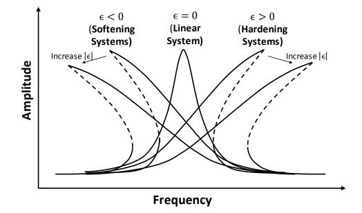
Figure 2.2. The amplitude-frequency response of Duffing resonator circuits with different nonlinearity coefficients ( $\epsilon$ ).
