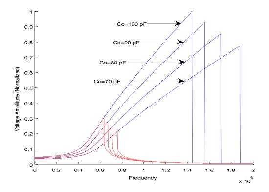
Figure 2.13. The frequency responses of the BST-based Duffing resonator circuits with different  $C_0$  (zero-bias capacitance) values. The solid blue curve shows the high-amplitude equilibrium points, while the solid red curve shows the low-amplitude equilibrium points.
