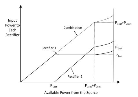
Figure 4.5. Ideal input power to Rectifier 1, Rectifier 2, and their combination, as functions of available power level.
