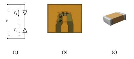
Figure 2.6. (a) Anti-series connected varactor diode pair, (b) an example of ferroelectric barium strontium titanate (BST) varactor, and (c) an example of ceramic capacitor: C2225C102KHRAC SMD
