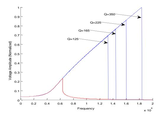
Figure 2.11. The frequency response of the Duffing resonator circuit for different Q values from 125 to 350. The solid blue curve shows the high-amplitude equilibrium points at different frequencies, while the solid red curve shows the low-amplitude equilibrium points.
