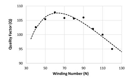
Figure 3.2. Measured Q (dots) of ferrite antenna versus the number of windings
