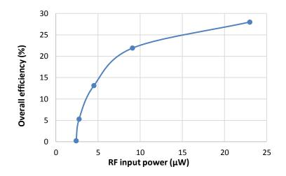
Figure 3.14. The overall RF-DC efficiency vs. RF input power levels of the WPH receiver
