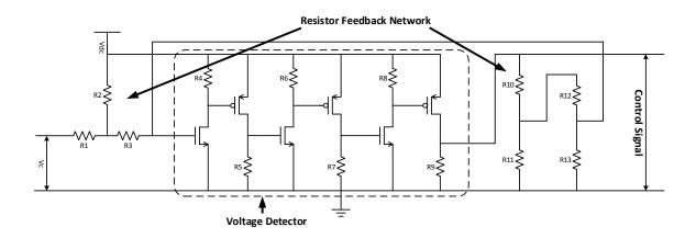
Figure 3.11. Schematic of the Schmitt Trigger Circuit, dashed box shows the voltage detector, the resistors outside the box provide positive feedback.
