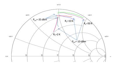
Figure 3.8. Optimum impedance matching condition versus input power at 900 MHz for  $R_L = 2 k\Omega$ , 10  $k\Omega$  and 50  $k\Omega$ . Solid curves show the calculated values, and dashed curves show the values optimized with Agilent ADS software. Smith Chart is normalized to  $Z_0 = 1 k\Omega$  for the convenience of plotting.
