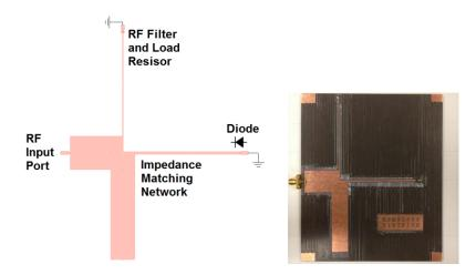
Figure 3.6. Shunt-connected diode rectifier with HSMS 2852 Schottky diode for a 900 MHz wireless power harvester
