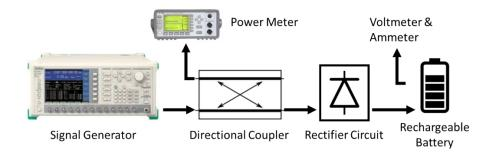
Figure 4.19. Measurement setup.
