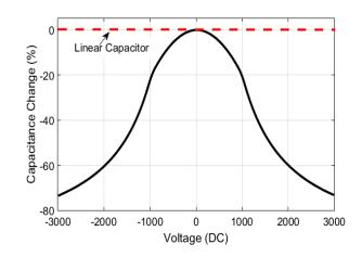
Figure 2.8. An example of nonlinear ceramic capacitors: tunability curve of a 3.0 kV, 1.0 nF multilayer ceramic commercial capacitor
