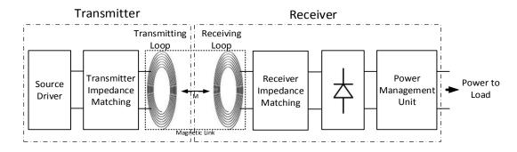
Figure 1.2. Block diagram of a typical two-coil SCMR WPT system
